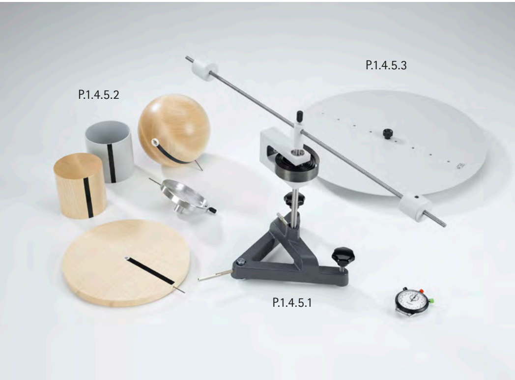
Definition of moment of inertia (P1.4.5.1)
