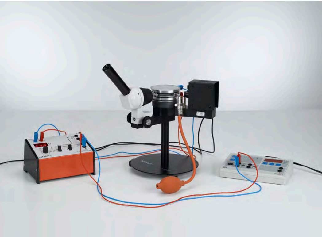
Determining the electric unit charge according to Millikan and verifying the charge quantification - Measuring the suspension voltage and the falling speed (P6.1.2.1)
