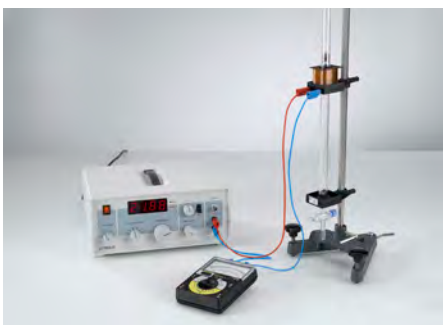
Determining the adiabatic exponent c_p/c_v of various gases using the gas elastic resonance apparatus (P2.5.3.2)
