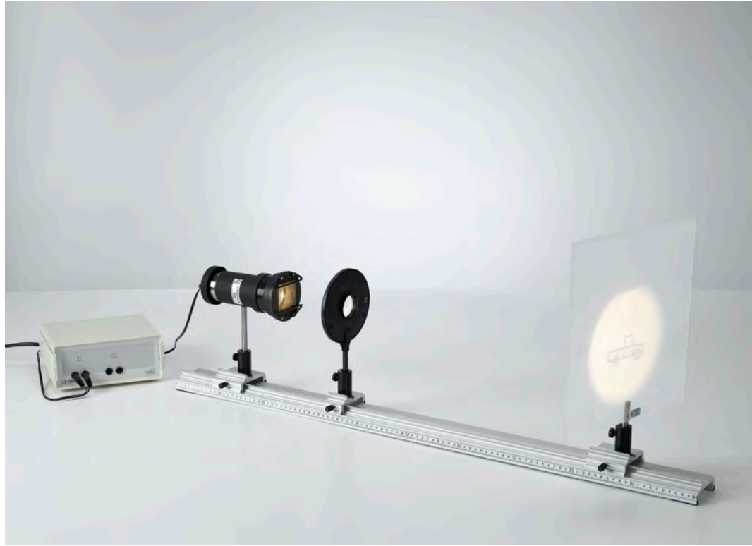
Verifying the imaging laws with a collecting lens (P5.1.2.4)
