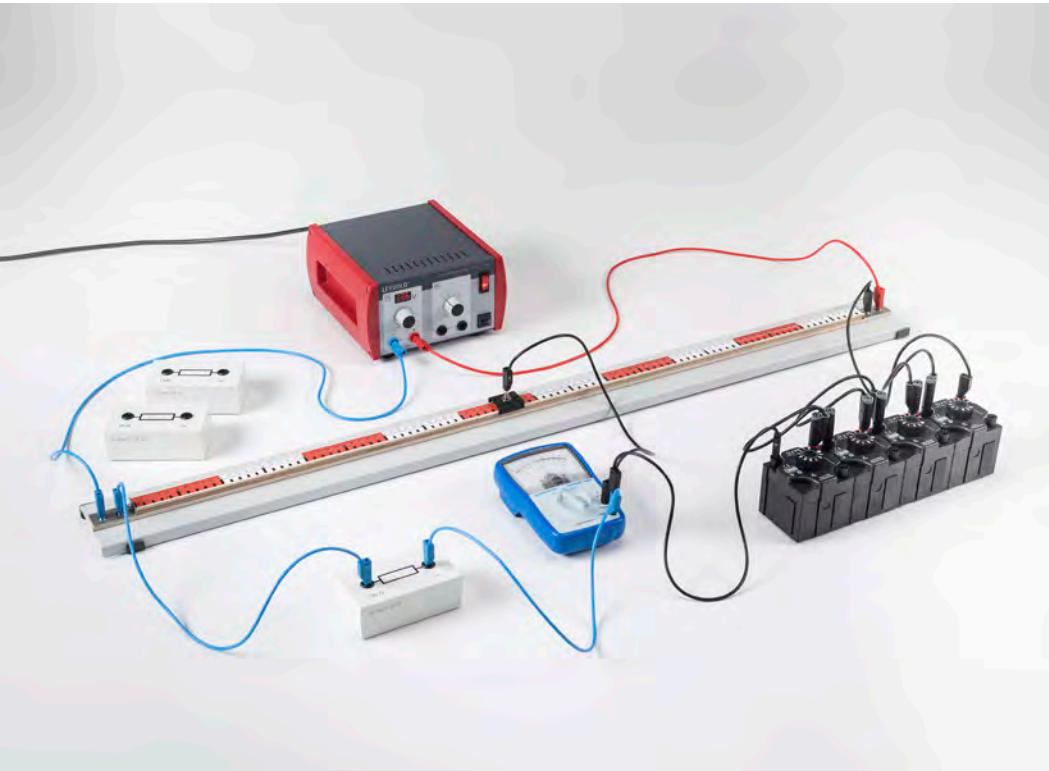
Determining resistances using a Wheatstone bridge (P3.2.3.4)
