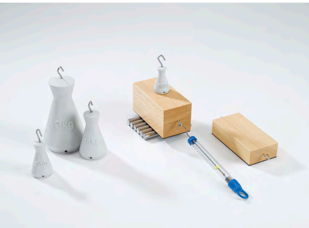
Static friction, sliding friction and rolling friction (P1.2.6.1)
