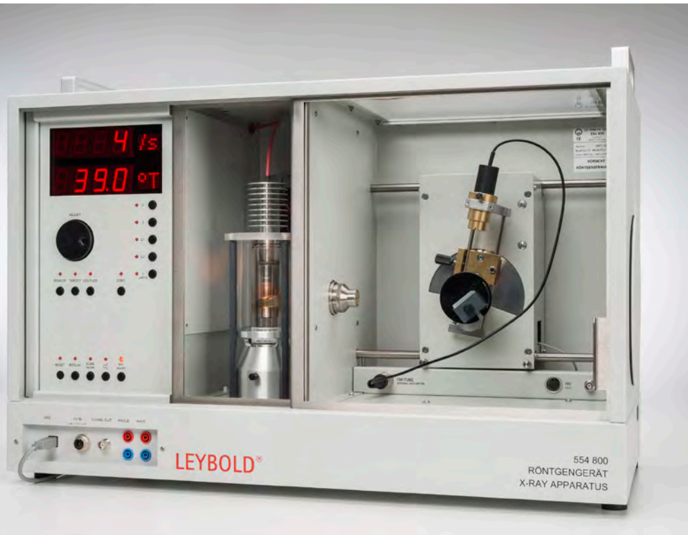
Fine structure of the characteristic X-ray radiation of a molybdenum anode (P6.3.6.1)
