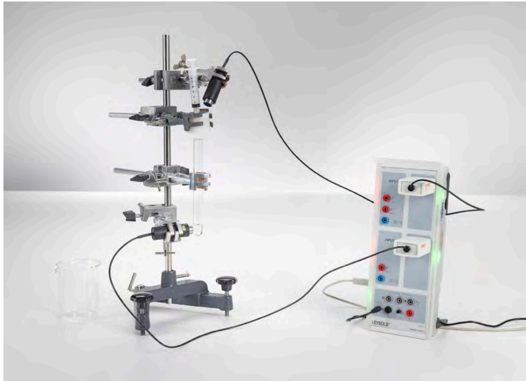
Determination of half-life of Cs-137 - Recording and evaluating the decay and production curve with CASSY (P6.4.3.4)
