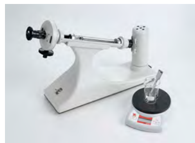
Determining the concentration of sugar solutions with a standard commercial polarimeter (P5.4.3.4)
