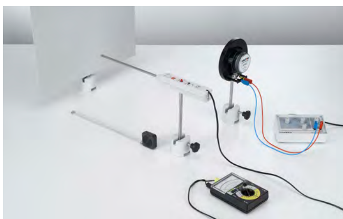
Determining the wavelength of standing sound waves (P1.7.3.2)
