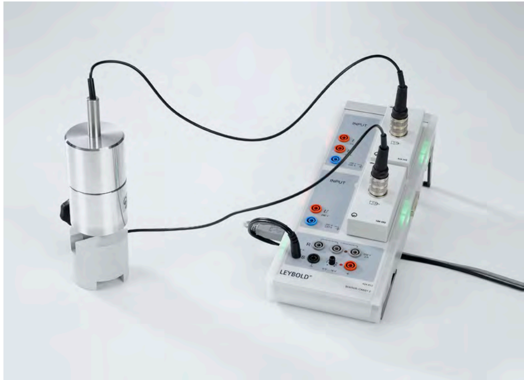
Detection of Muons (P6.6.2.1)
