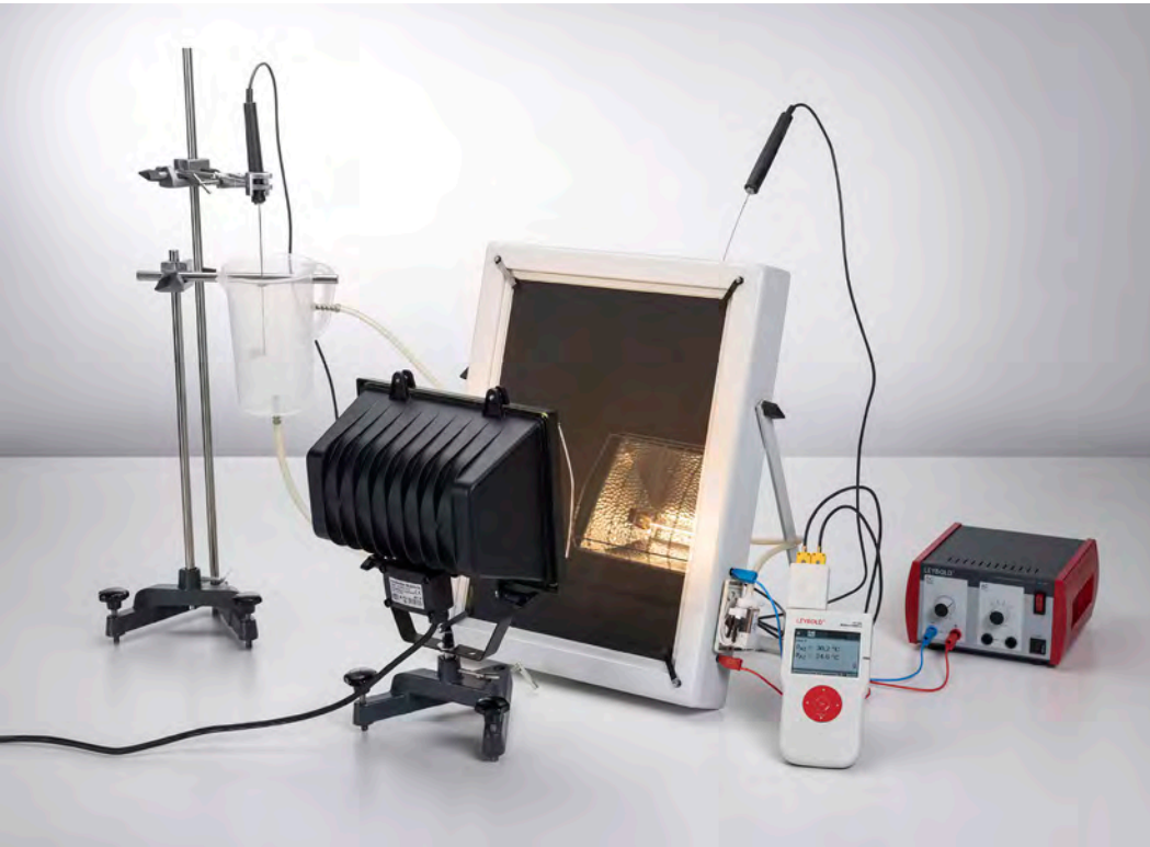
Efficiency of a solar collector (P2.2.2.1)
