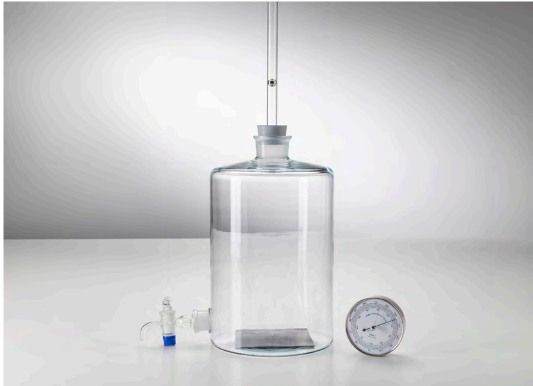
Determining the adiabatic exponent c_p/c_v of air according to Rüchardt (P2.5.3.1)
