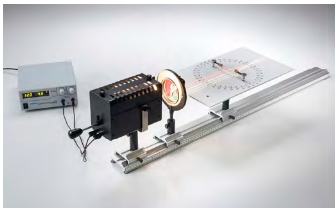
Refraction of light at straight surfaces and investigation of ray paths in prisms and lenses (P5.1.1.2)
