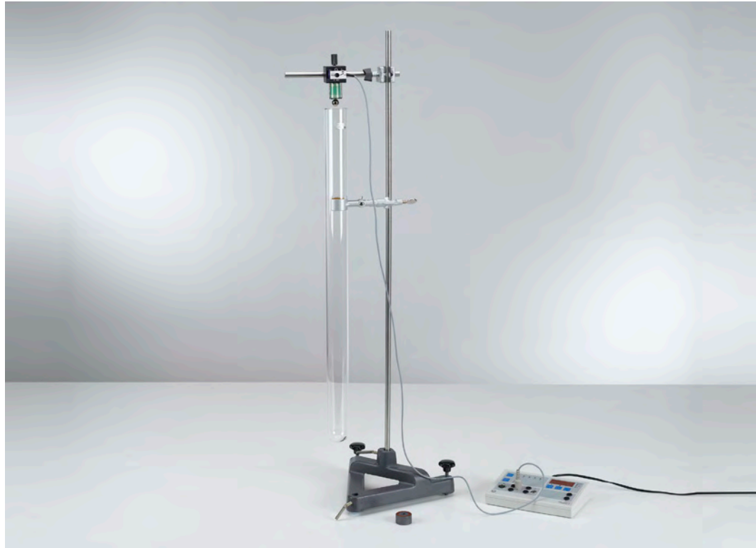
Assembling a falling-ball viscosimeter to determine the viscosity of viscous fluids (P1.8.3.1)
