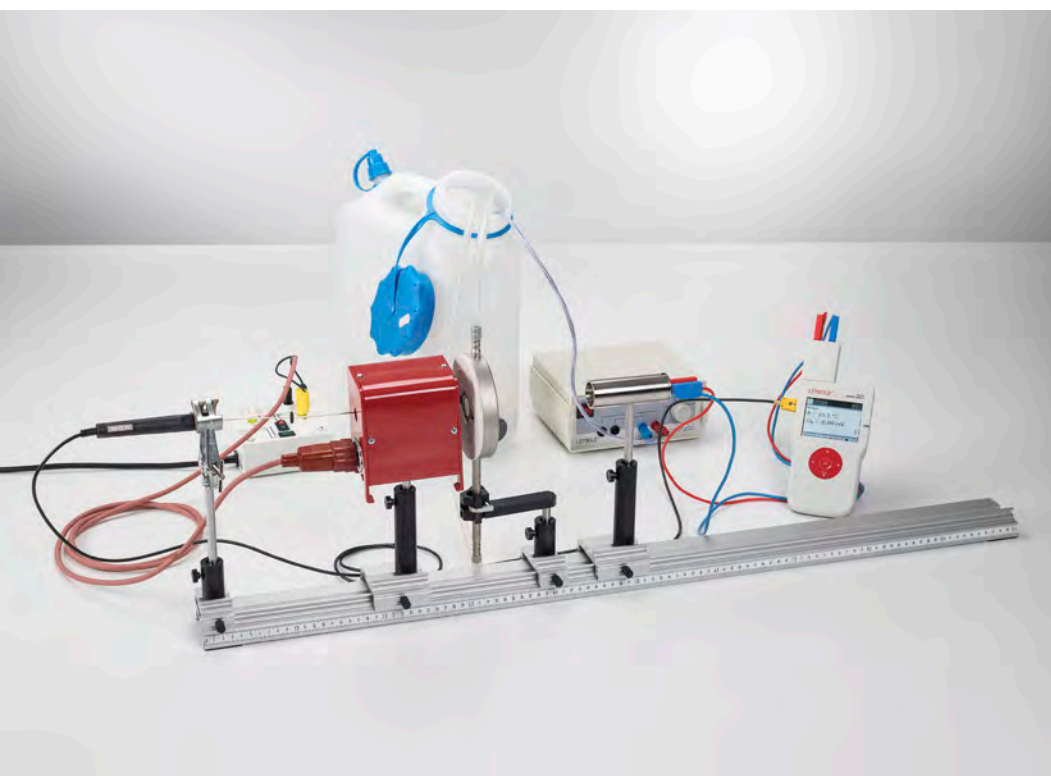
Stefan-Boltzmann law: measuring the radiant intensity of a „black body“ as a function of temperature (P5.5.2.1)
