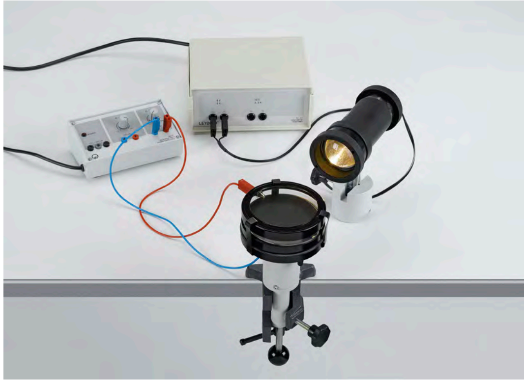
Demonstrating the tracks of \alpha particles in a Wilson cloud chamber (P6.5.1.1)
