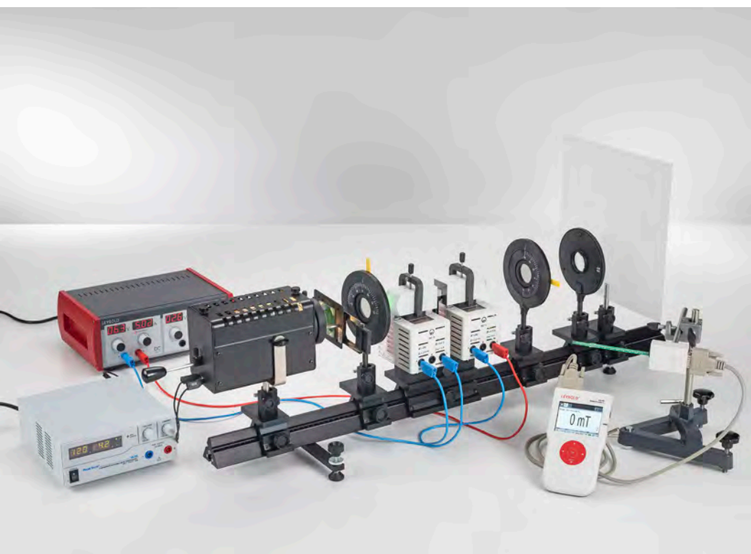
Faraday effect: determining Verdet's constant for flint glass as a function of the wavelength (P5.4.6.1)
