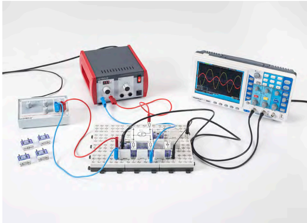
The field-effect transistor as an amplifier (P4.1.6.5)
