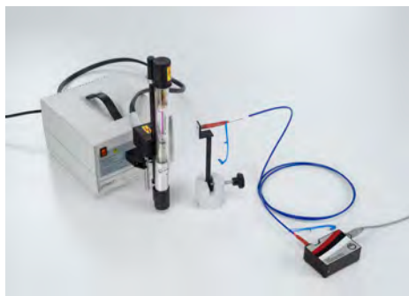
Emission spectrum of atomic hydrogen (P6.2.1.4)
