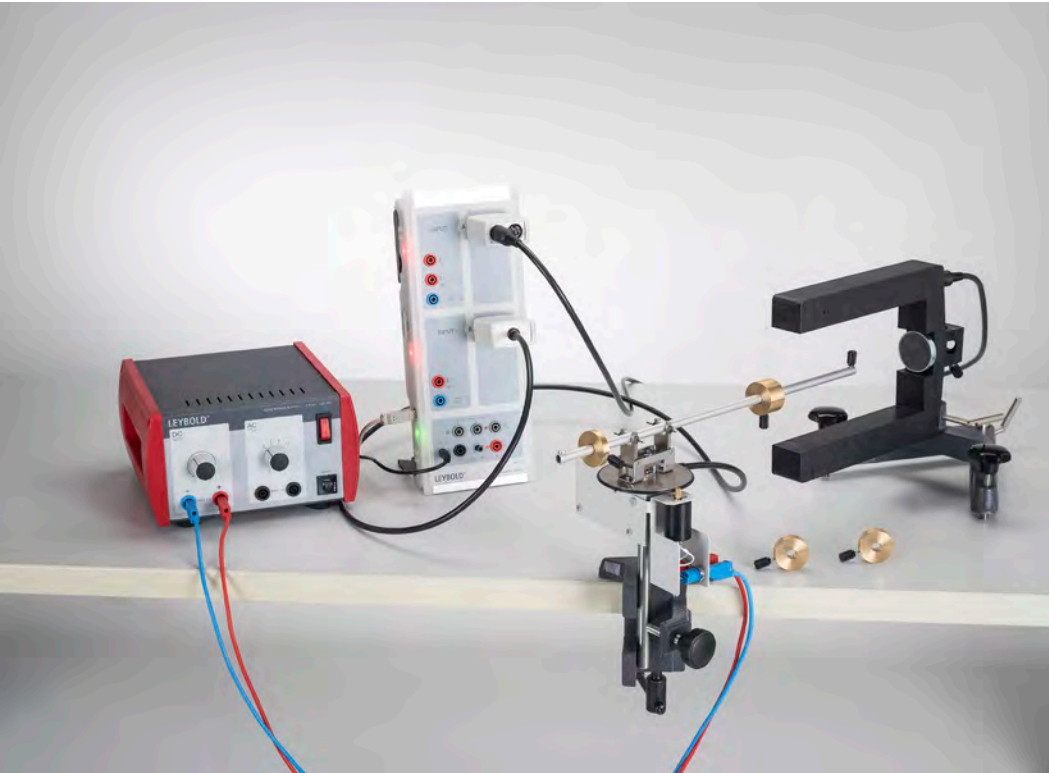
Centrifugal force of an orbiting body - Measuring with the central force apparatus and CASSY (P1.4.3.3)
