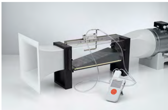
Verifying the Bernoulli equation - Measuring with a pressure sensor and Mobile-CASSY (P1.8.7.4)
