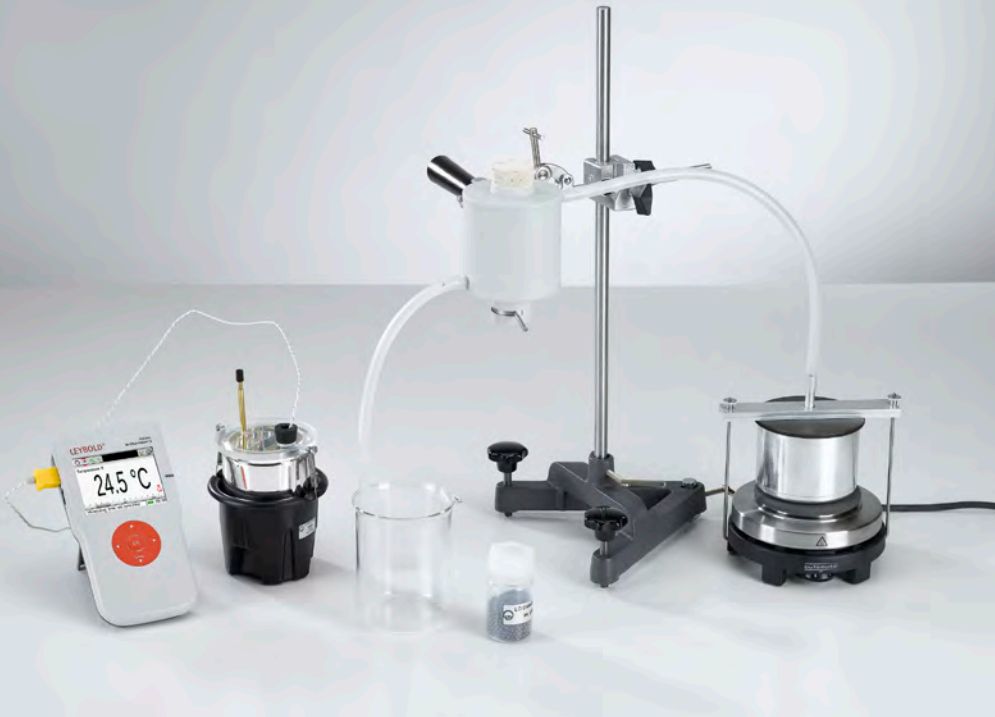
Determination of specific heat of solids - Measuring with Mobile-CASSY (P2.3.2.2)
