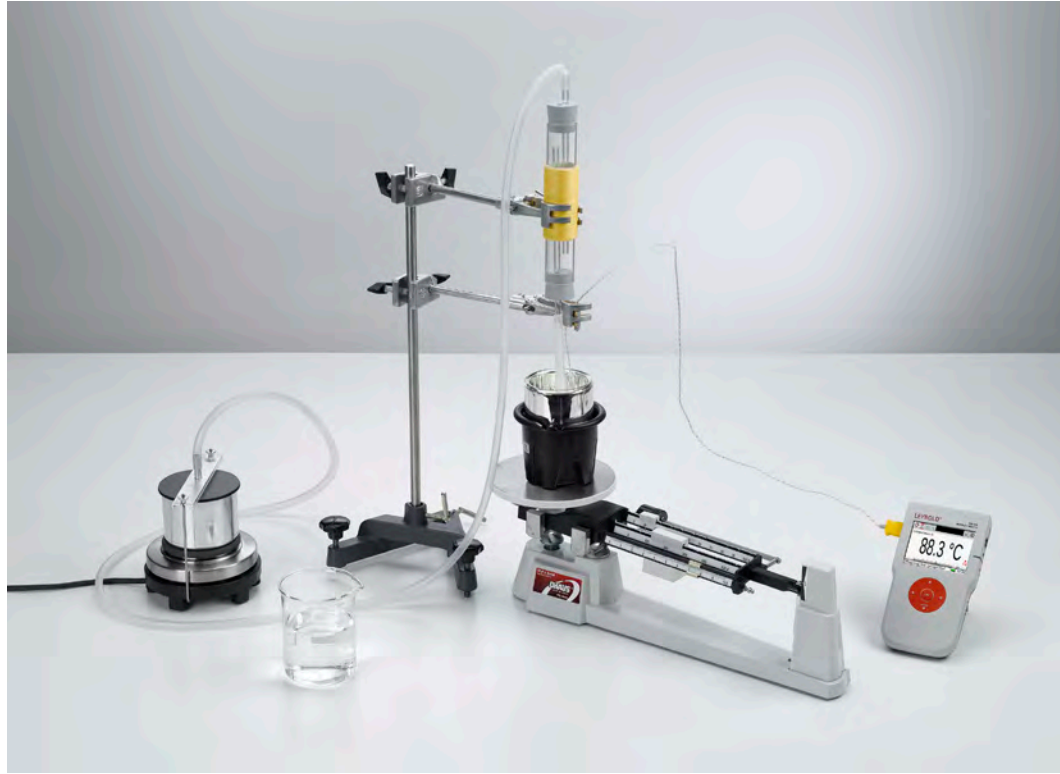
Determination of specific vaporization heat of water - Measuring with Mobile-CASSY (P2.4.1.3)
