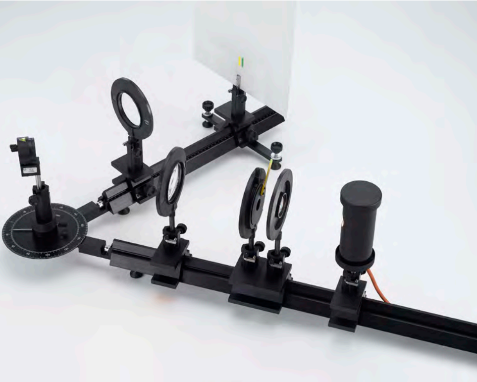
Investigating the spectrum of a high pressure mercury lamp (P6.2.2.3)
