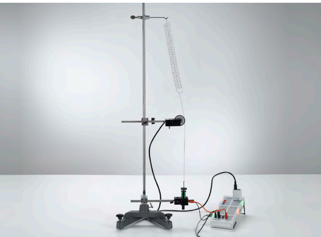
Oscillations of a spring pendulum and determination of oscillation period as a function of the oscillating mass - Measuring with CASSY (P1.5.2.1)
