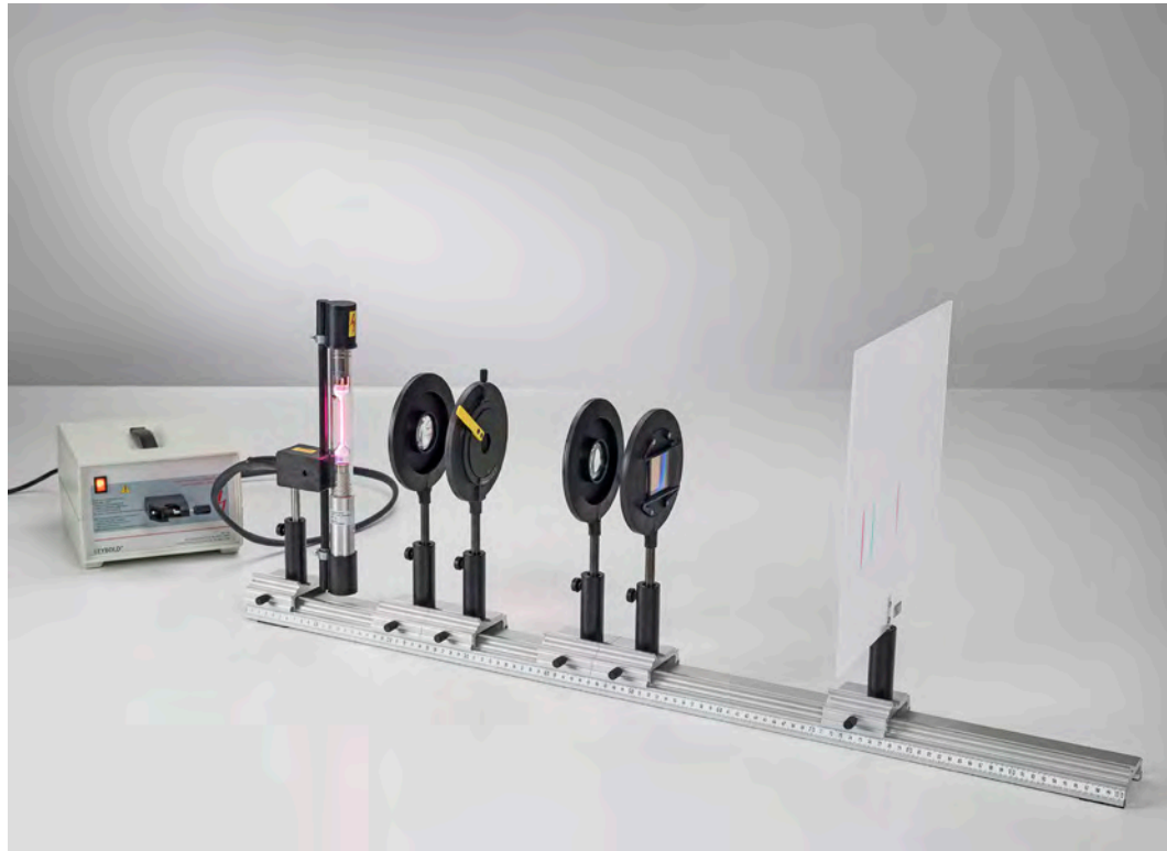
Determining the wavelengths H_\alpha , H_\beta and H_\gamma from the Balmer series of hydrogen (P6.2.1.1)
