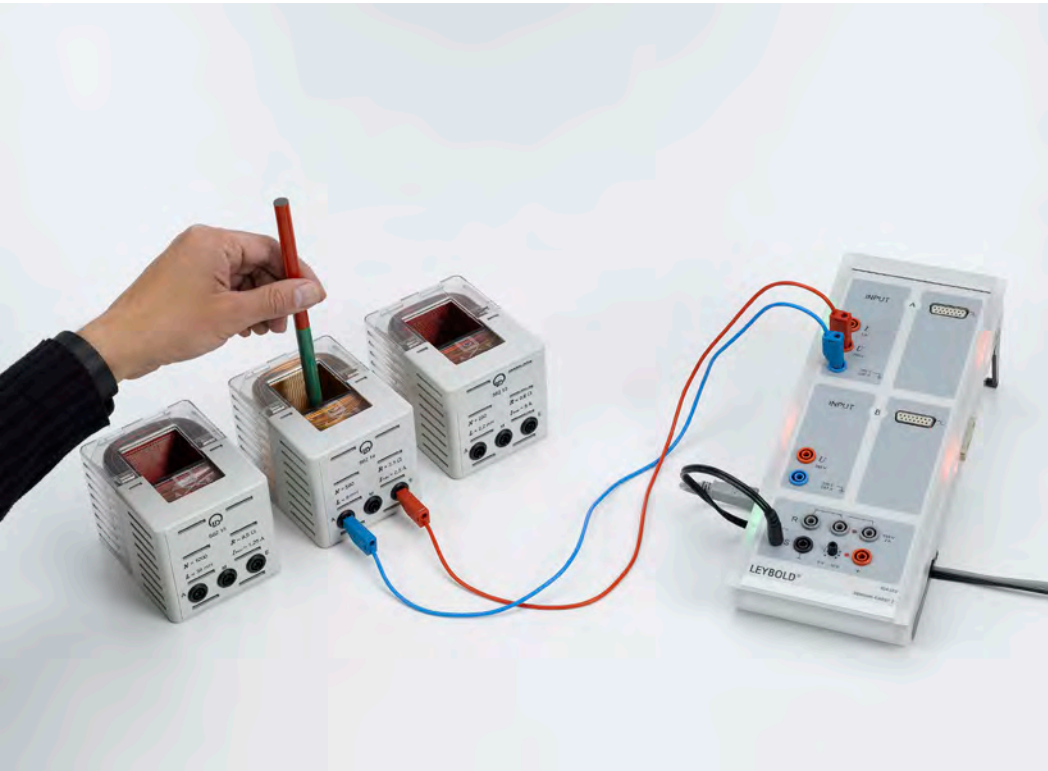
Generating a voltage surge in a conductor loop with a moving permanent magnet (P3.4.1.1)
