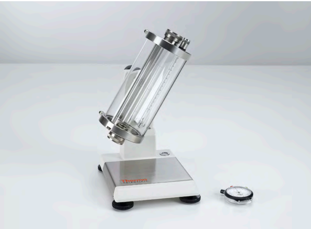
Falling-ball viscosimeter: measuring the viscosity of sugar solutions as a function of the concentration (P1.8.3.2)
