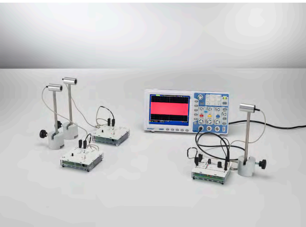
Beating of ultrasonic waves (P1.7.5.1)
