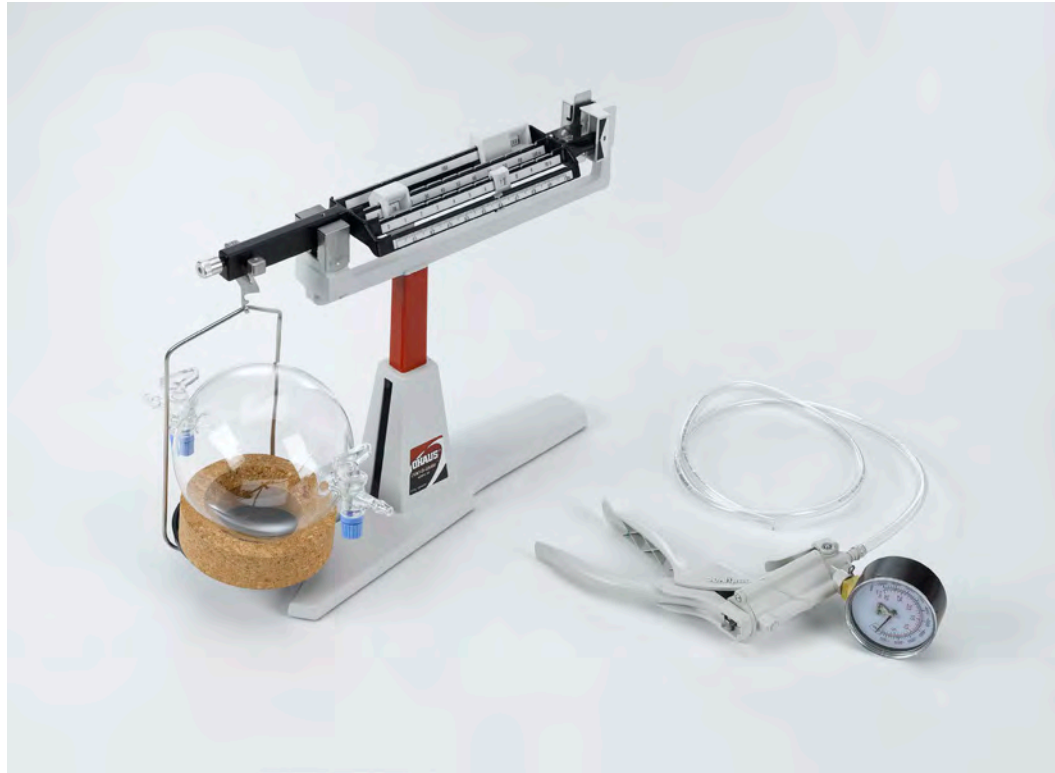
Determining the density of air (P1.1.2.4)
