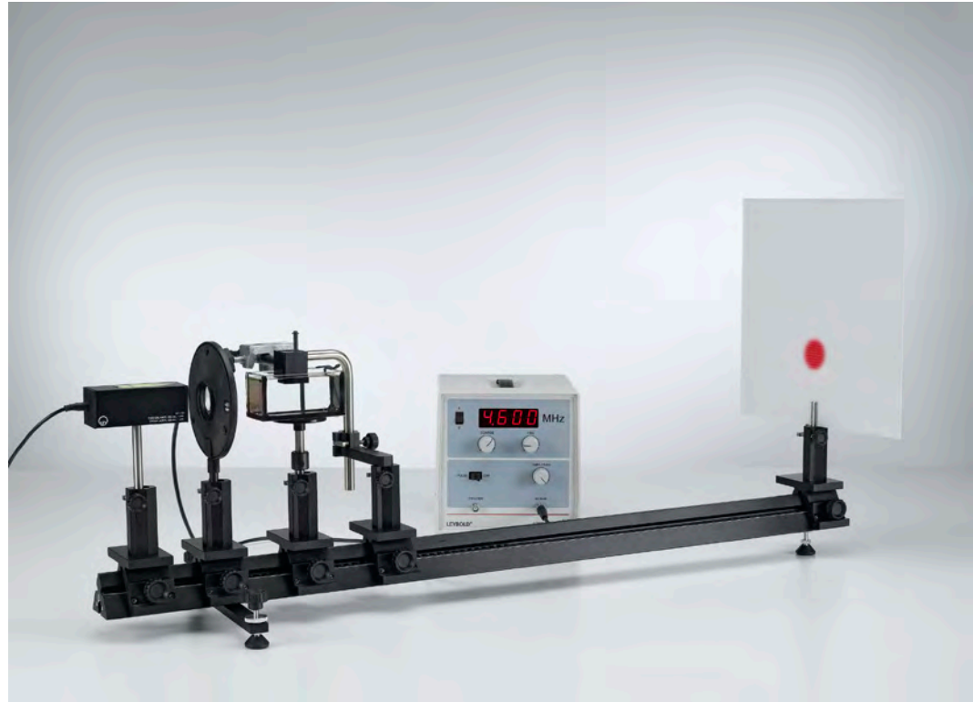
Determination of the velocity of sound in liquids - standing ultrasonic waves as optical grating (P1.7.8.1)
