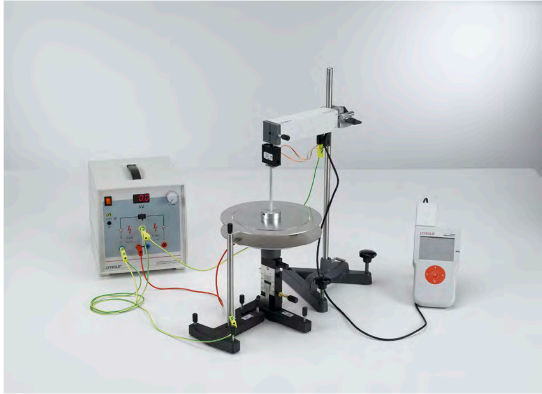
Kirchhoff's voltage balance: Measuring the force between two charged plates of a plate capacitor - Measuring with the force sensor (P3.1.4.2)
