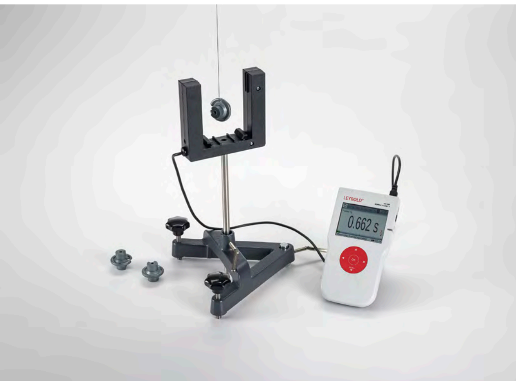
Determination of gravitational acceleration with a simple pendulum - Measuring with light barrier (P1.5.1.7)
