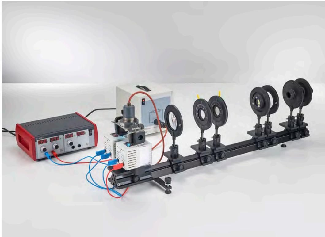
Observing the normal Zeeman effect in transverse and longitudinal configuration - spectroscopy using a Fabry-Perot etalon (P6.2.7.3)
