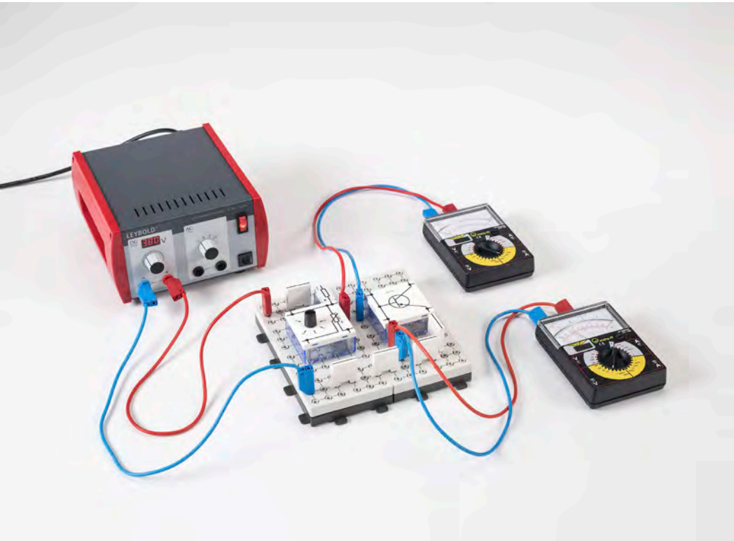
Recording the characteristics of a transistor (P4.1.5.2)
