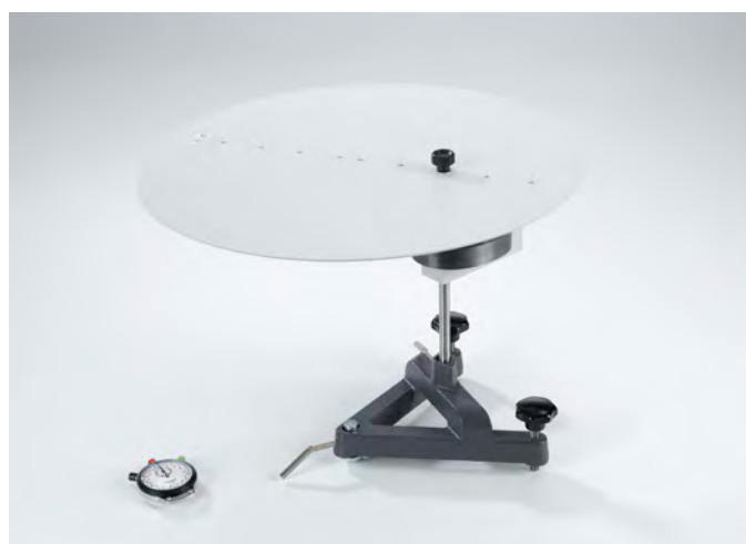
Confirming Steiner's theorem (P1.4.5.3)
