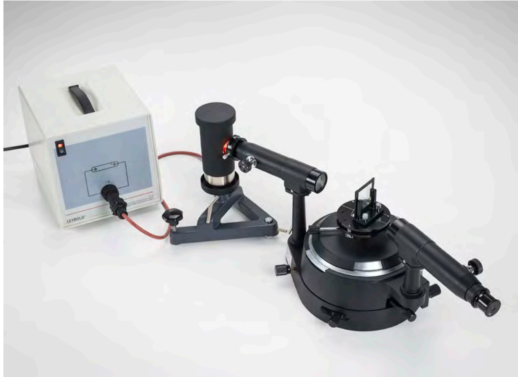
Measuring the line spectra of inert gases and metal vapors using a grating spectrometer (P5.7.2.1)
