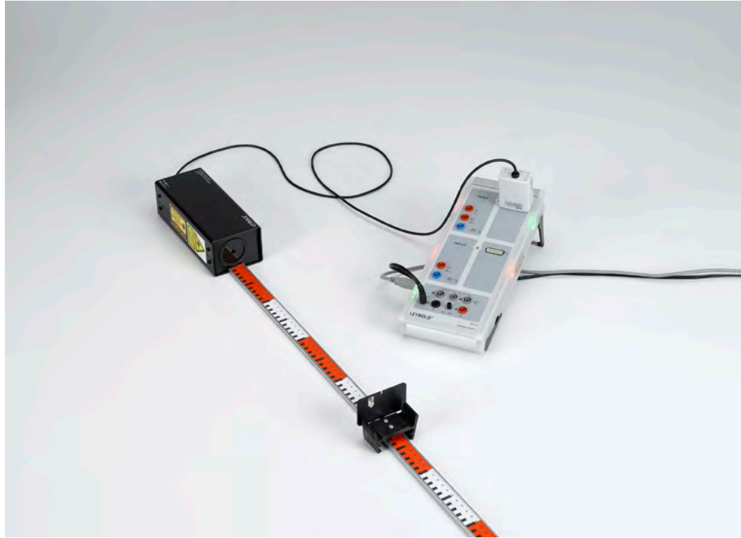
Determining the velocity of light using a periodical light signal at a short measuring distance - measuring with the laser motion sensor S and CASSY (P5.6.3.3)
