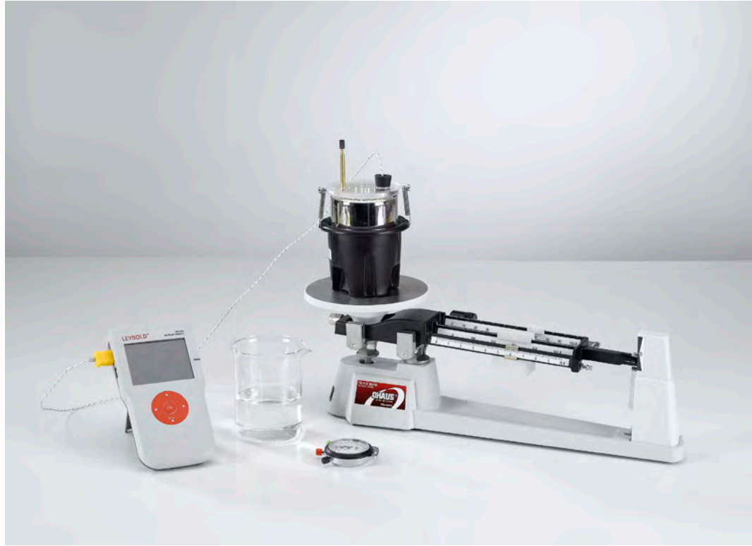
Mixing temperature of water - Measuring with Mobile-CASSY (P2.3.1.2)
