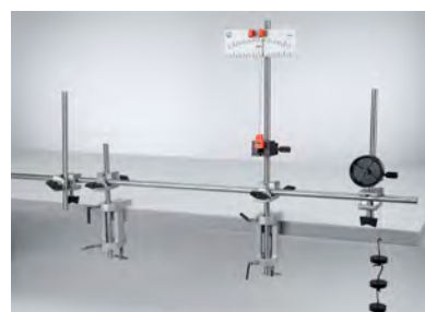
Investigating the elastic and plastic extension of metal wires (P7.1.4.1)
