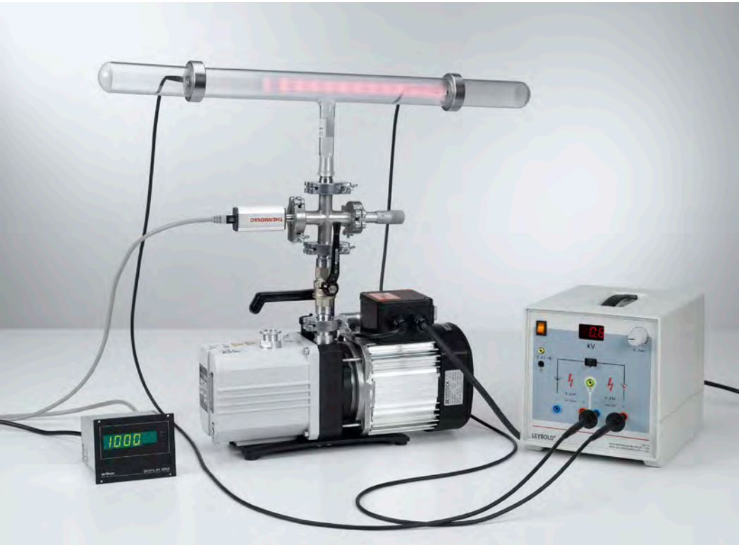
Investigating spontaneous gas discharge in air as a function of pressure (P3.9.2.1)
