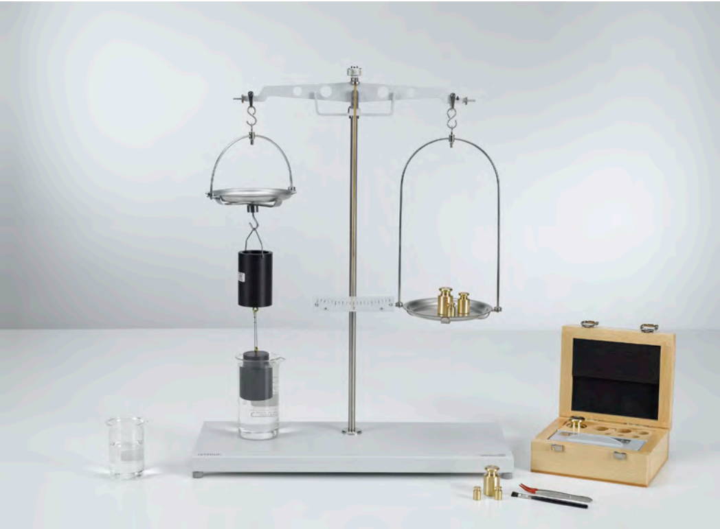
Confirming Archimedes' principle (P1.8.2.1)
