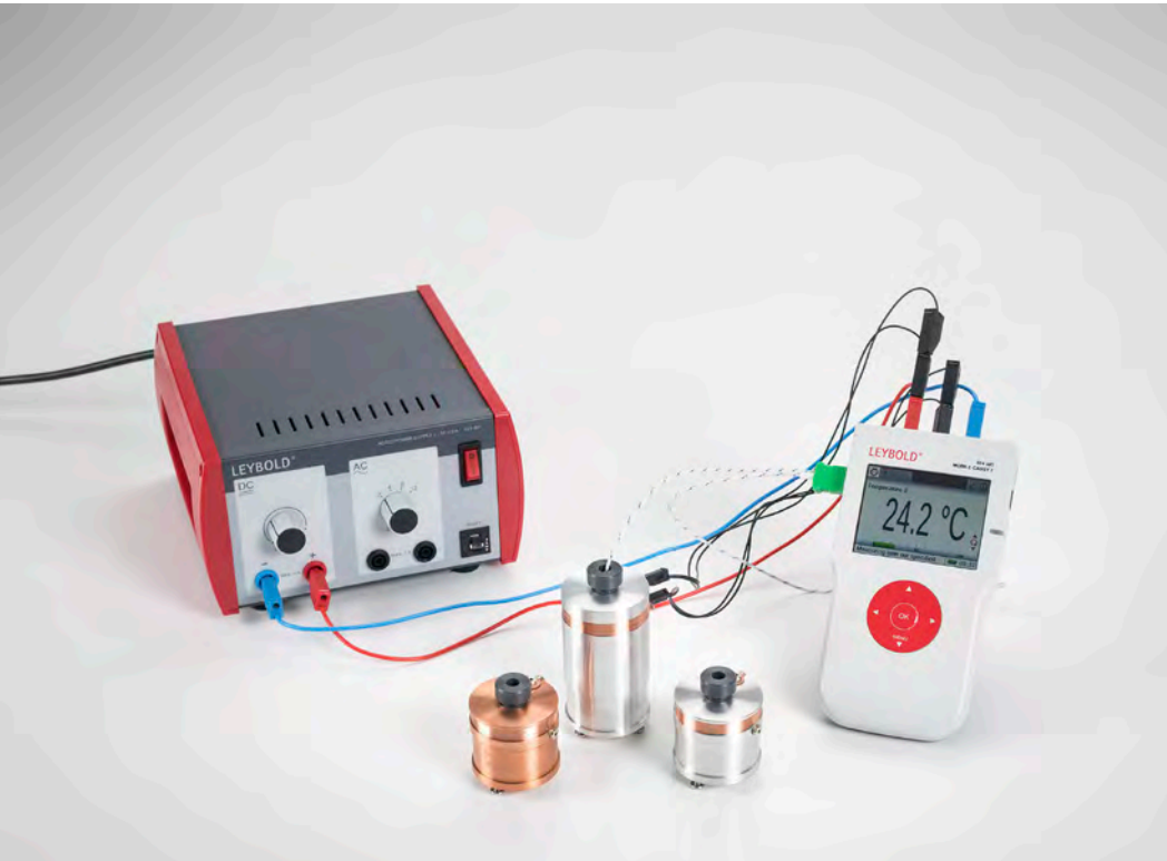
Converting electrical energy into heat energy - Measuring with Mobile-CASSY (P2.3.4.4)
