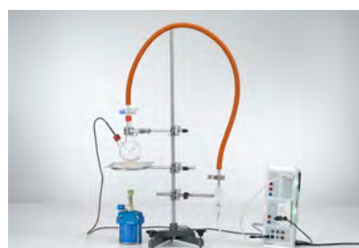
Recording the vapor-pressure curve of water - Pressures up to 1 bar (P2.4.2.1)
