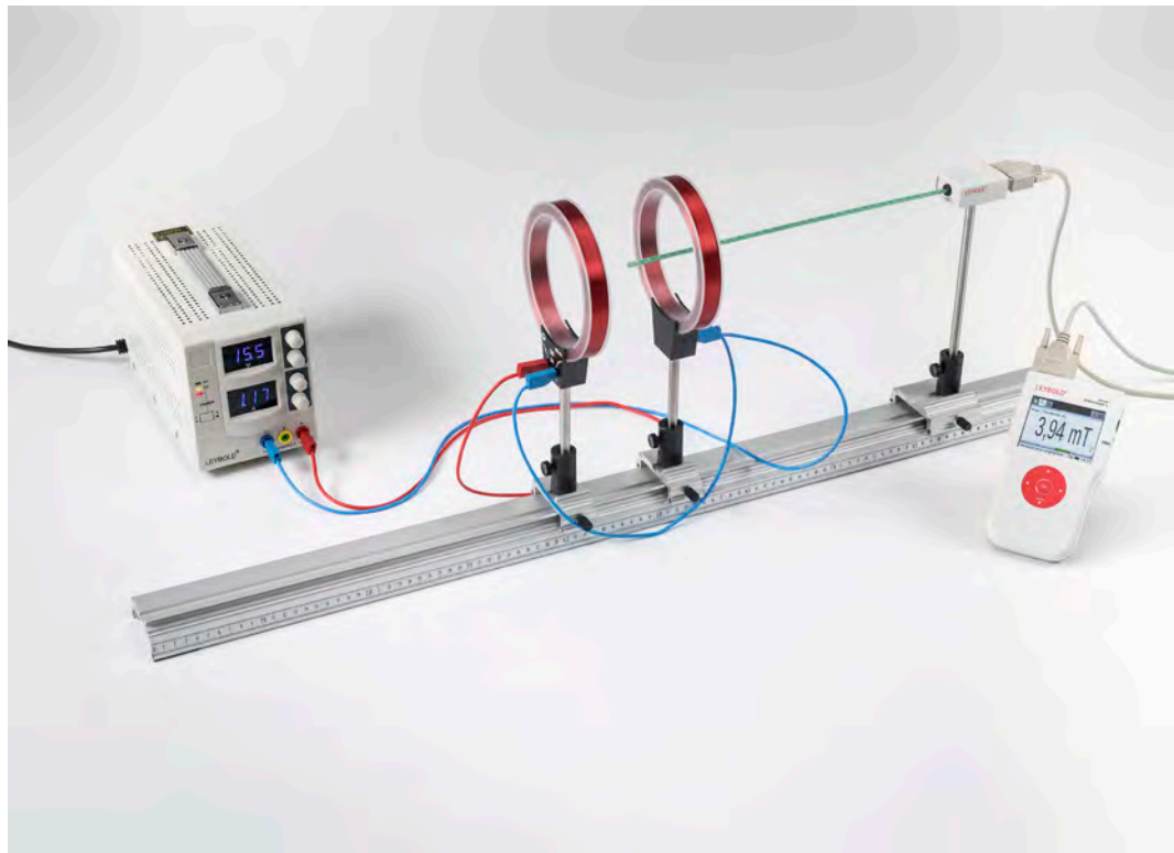
Measuring the magnetic field of a pair of coils in the Helmholtz configuration (P3.3.4.3)
