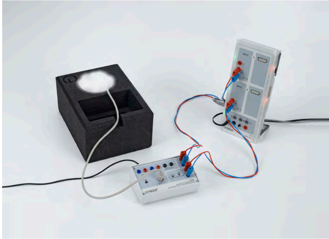
Determining the transition temperature of a high-temperature superconductor (P7.2.6.1)
