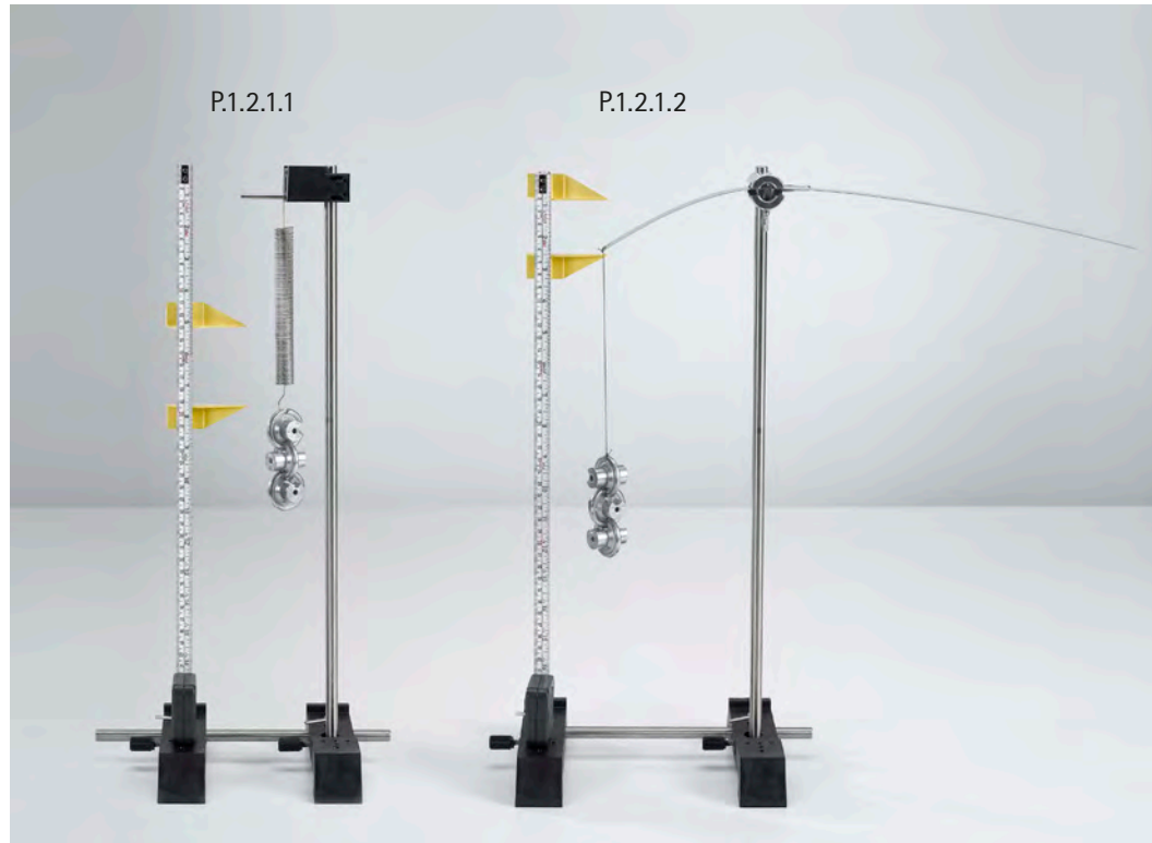
Expansion of a helical spring (P1.2.1.1)
