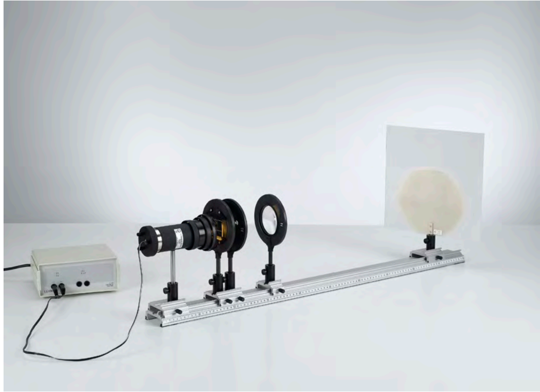
Magnifier and microscope (P5.1.4.1)
