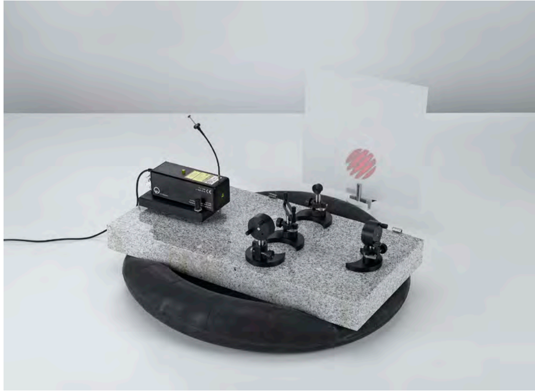
Setting up a Michelson interferometer on the laser optics base plate (P5.3.4.1)
