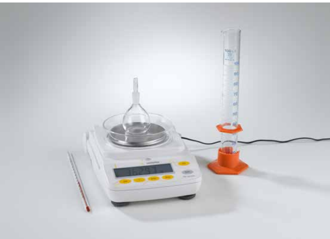
Determination of density with the pycnometer (C3.1.2.4)
