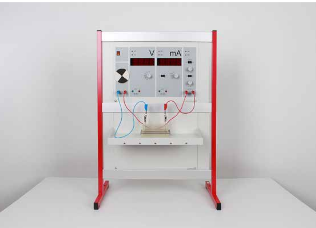
Conductivity of aqueous solutions (C4.4.1.7)
