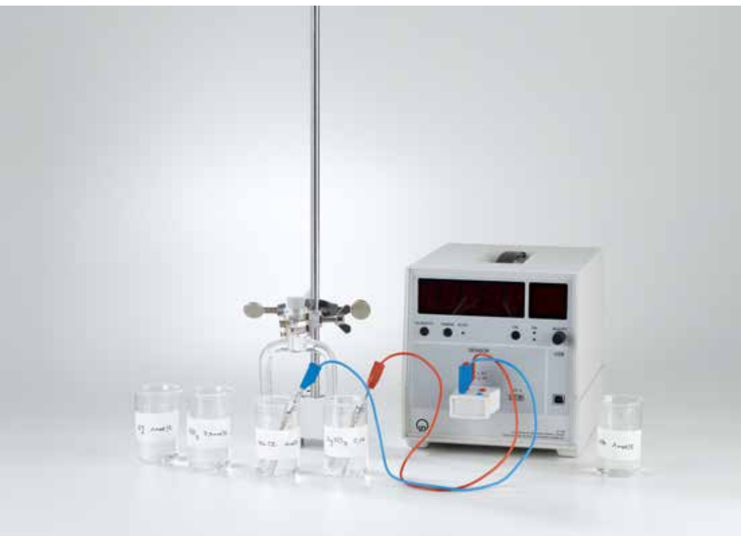
Determination of the complex disintegration constant of Silver diamine complex. (C4.2.3.1)
