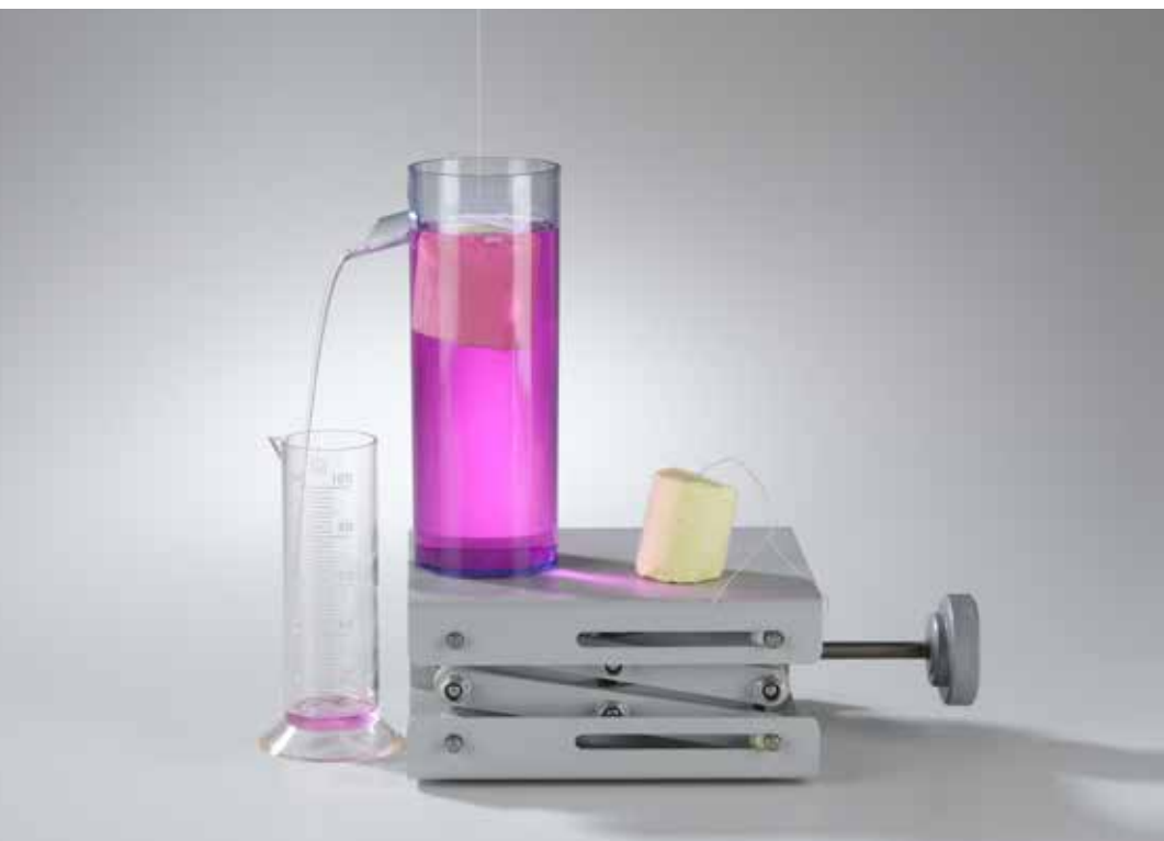
Determination of the density of solids (C3.1.3.4)
