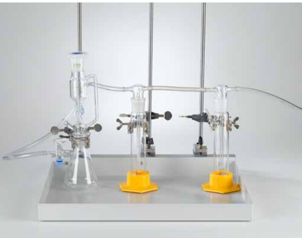
Production of gases with a dropping funnel (C1.4.2.2)
