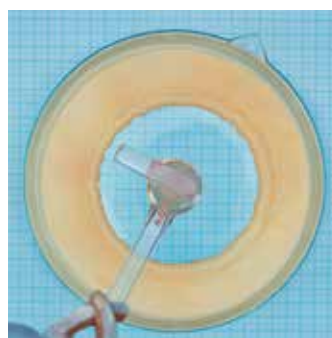
Determining the area A of the oil spot
