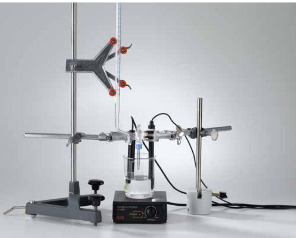
Conductometric titration of a hydrochloric acid solution with pH measurement (C3.5.2.2)
