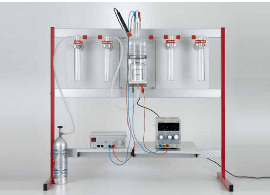
Determination of the heat of combustion of benzoic acid (C4.3.3.1_p)
