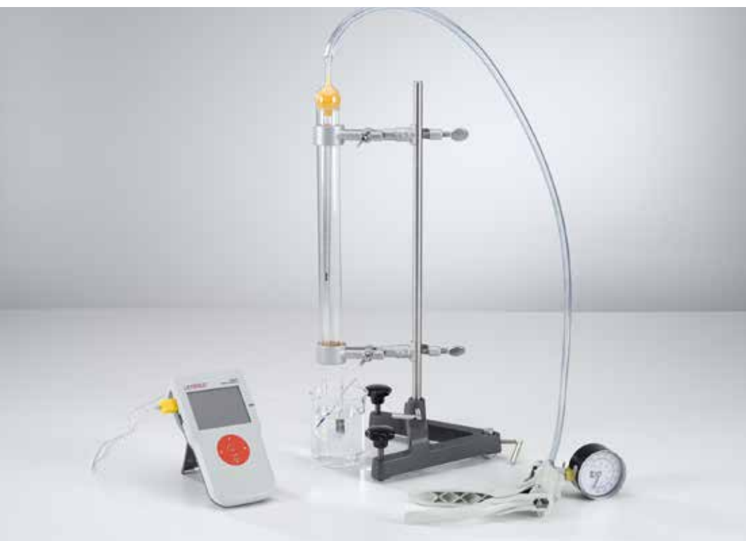
Temperature-dependency of the pressure of a gas at a constant volume (Amontons' law) (C1.4.4.3)
