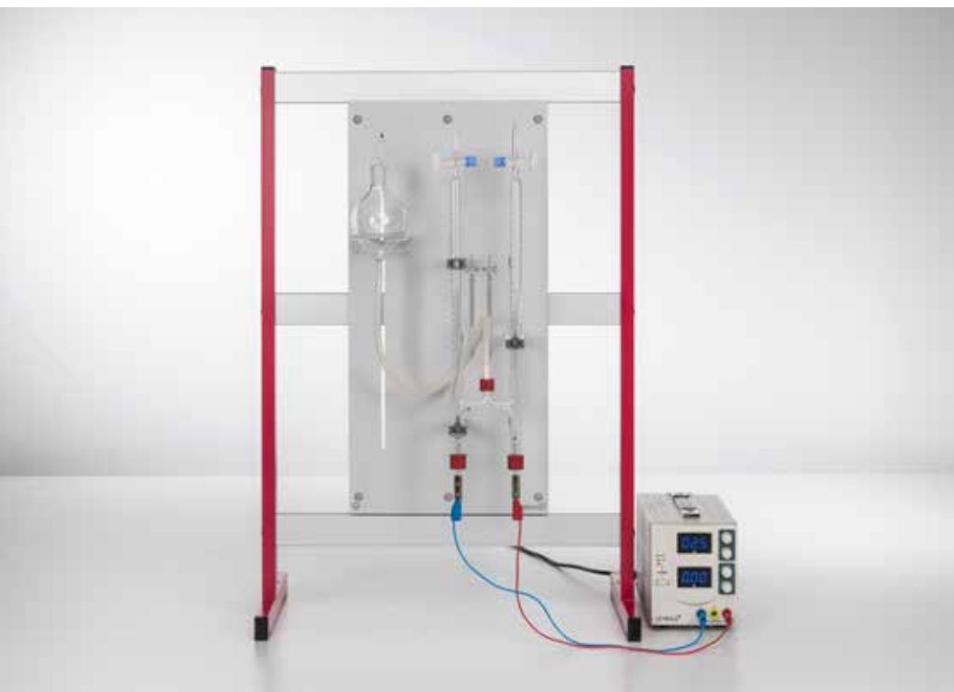
Electrolytic water decomposition according to Hoffmann (C1.3.1.1_p)
