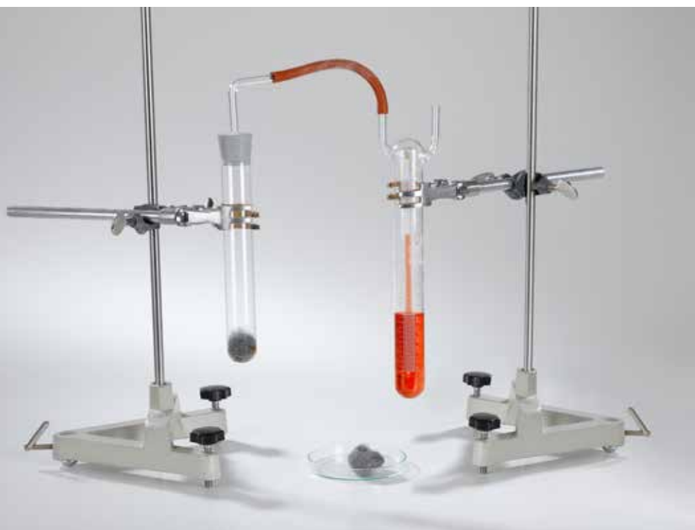
Conditions for iron corrosion (C1.5.3.1)
