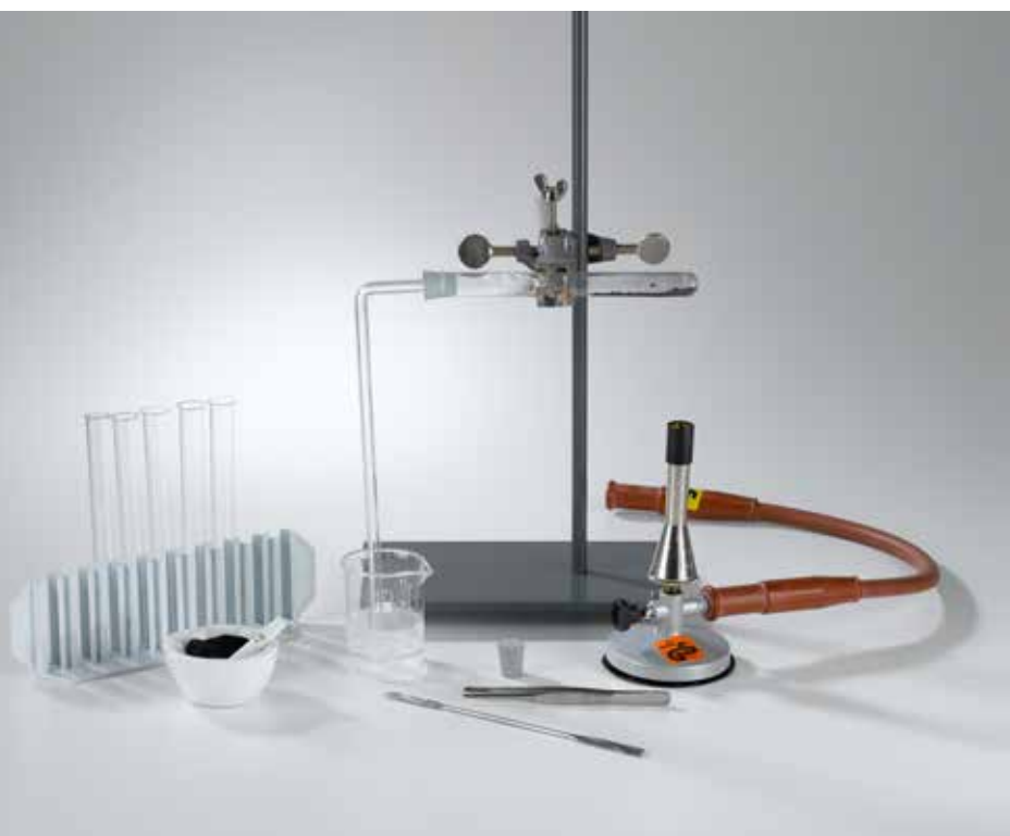
Extraction of copper from copper oxide (C1.5.1.1)
