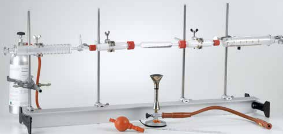
Quantitative determination of carbon (C2.1.1.1)
