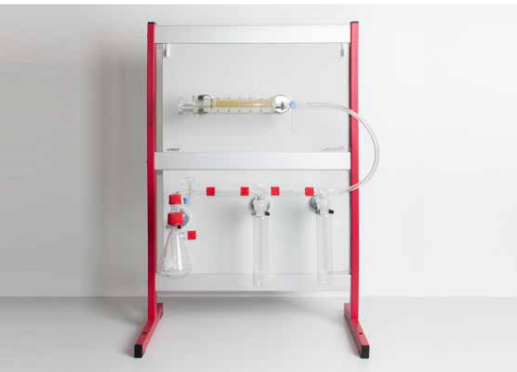
Production of gases with a Kipp's apparatus, CPS version (C1.4.2.1_p)
