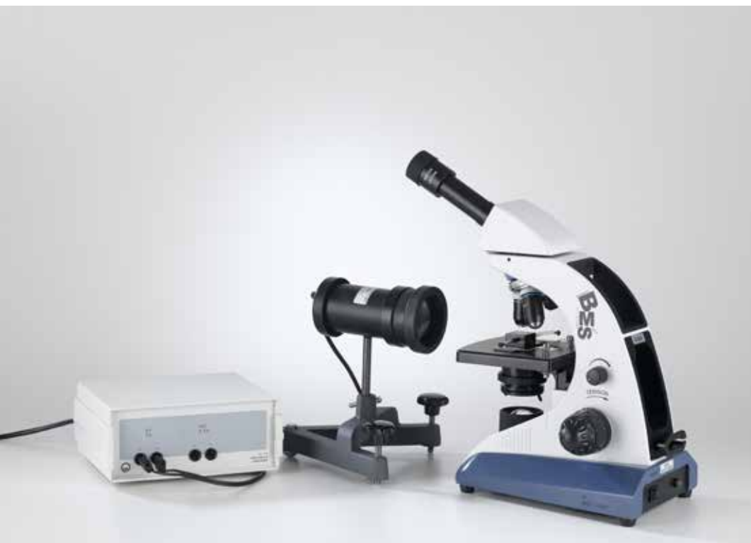
Brownian motion of smoke particles (C1.1.3.1)
