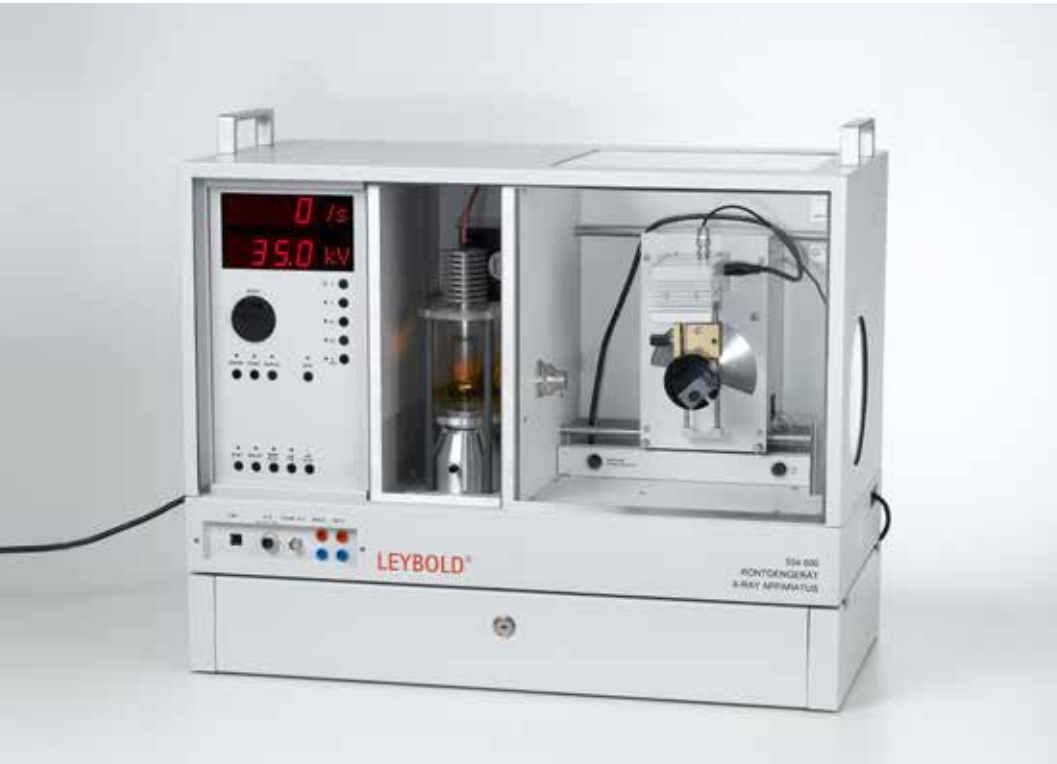
X-ray fluorescence analysis of chemical composition (C3.6.5.1)
