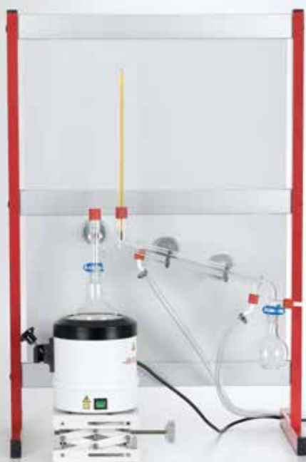
Purification of a substance with water vapour distillation (C2.4.3.3)
