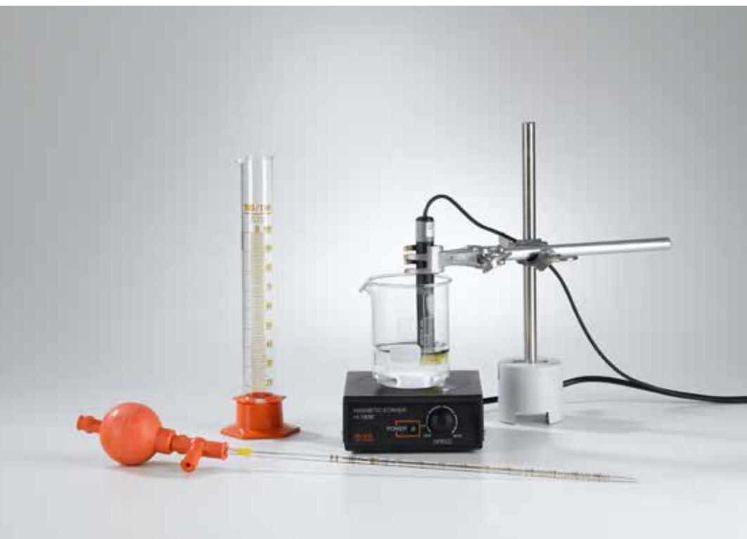
Hydrolysis of tertiary butyl chloride (C4.1.2.1)
