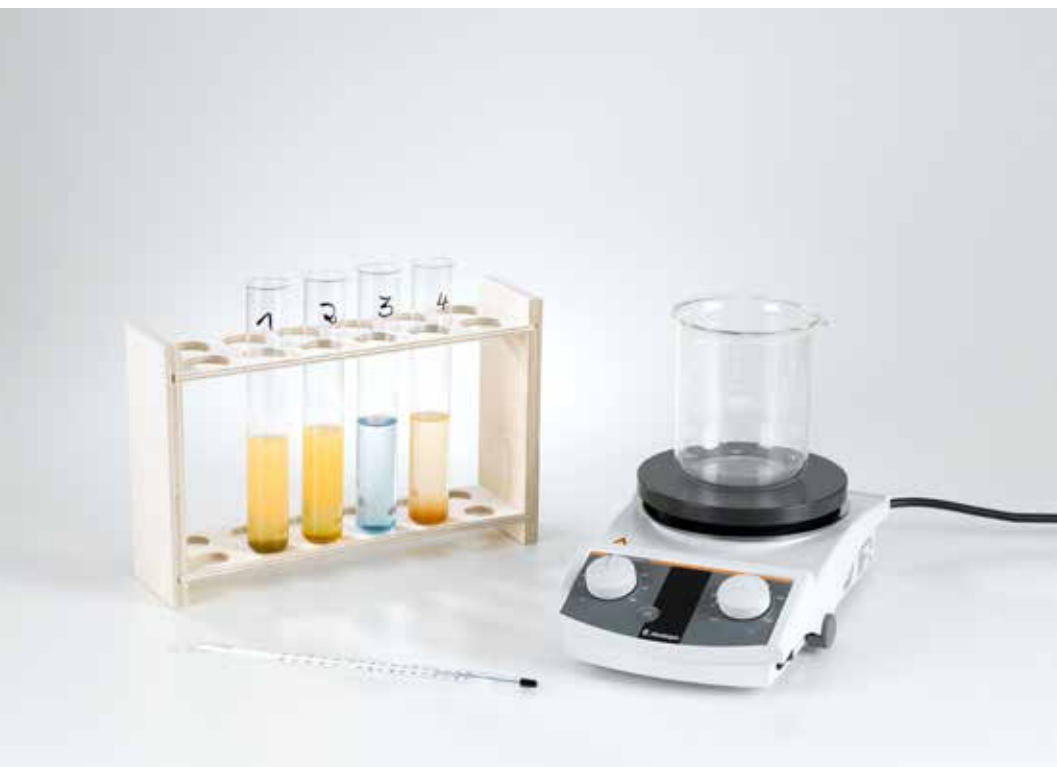
Test for reducing sugar - Fehling's reaction (C6.1.1.1)
