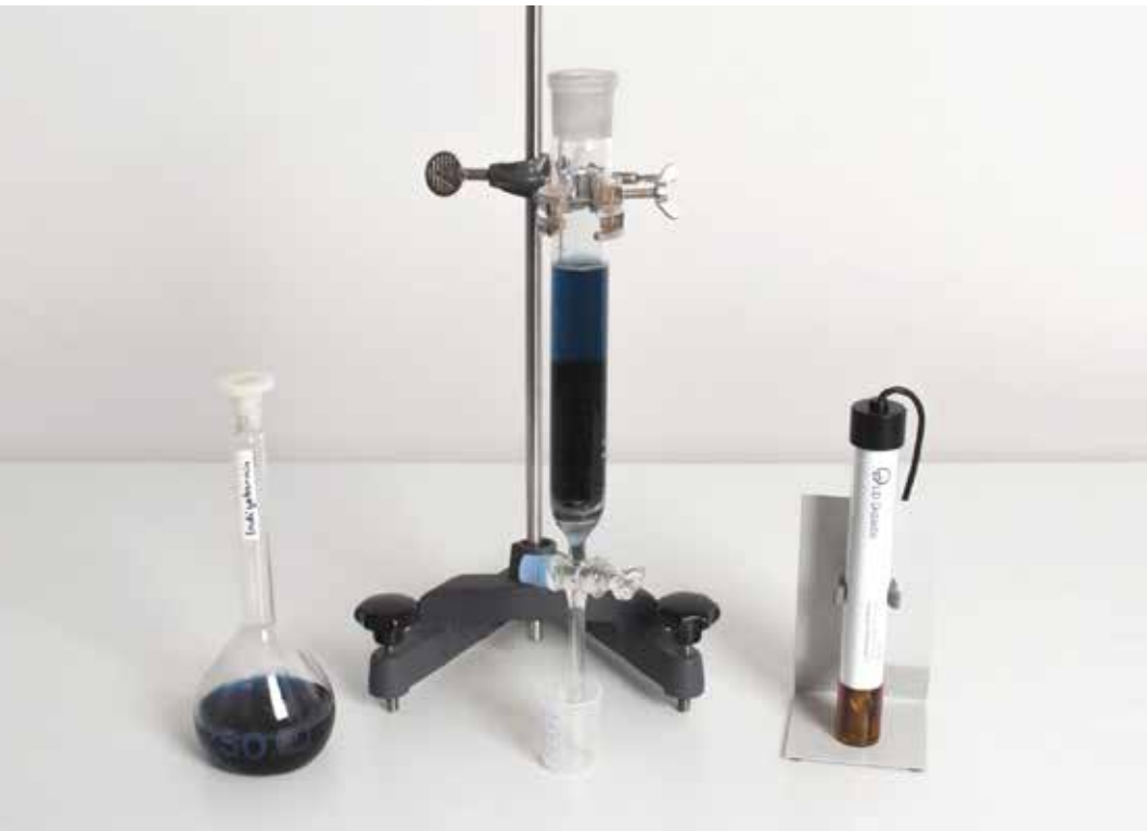
Recording a breakthrough curve of activated carbon filters (C5.3.3.1)
