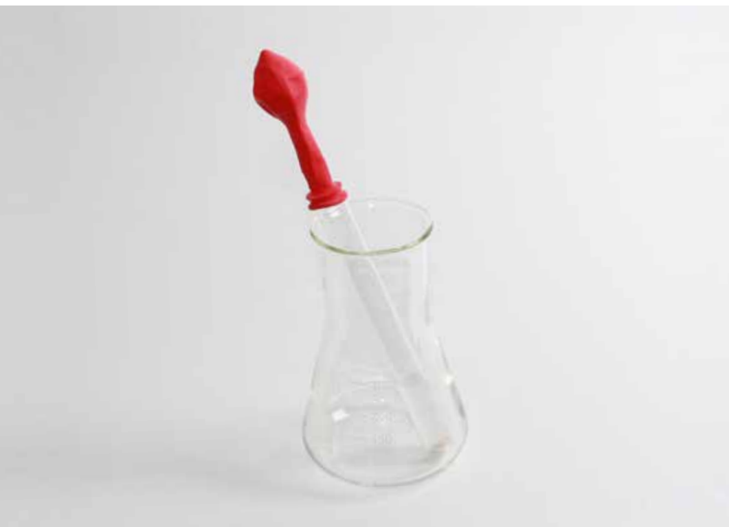
Conservation of mass in the reaction of marble with acid (C1.2.1.1)
