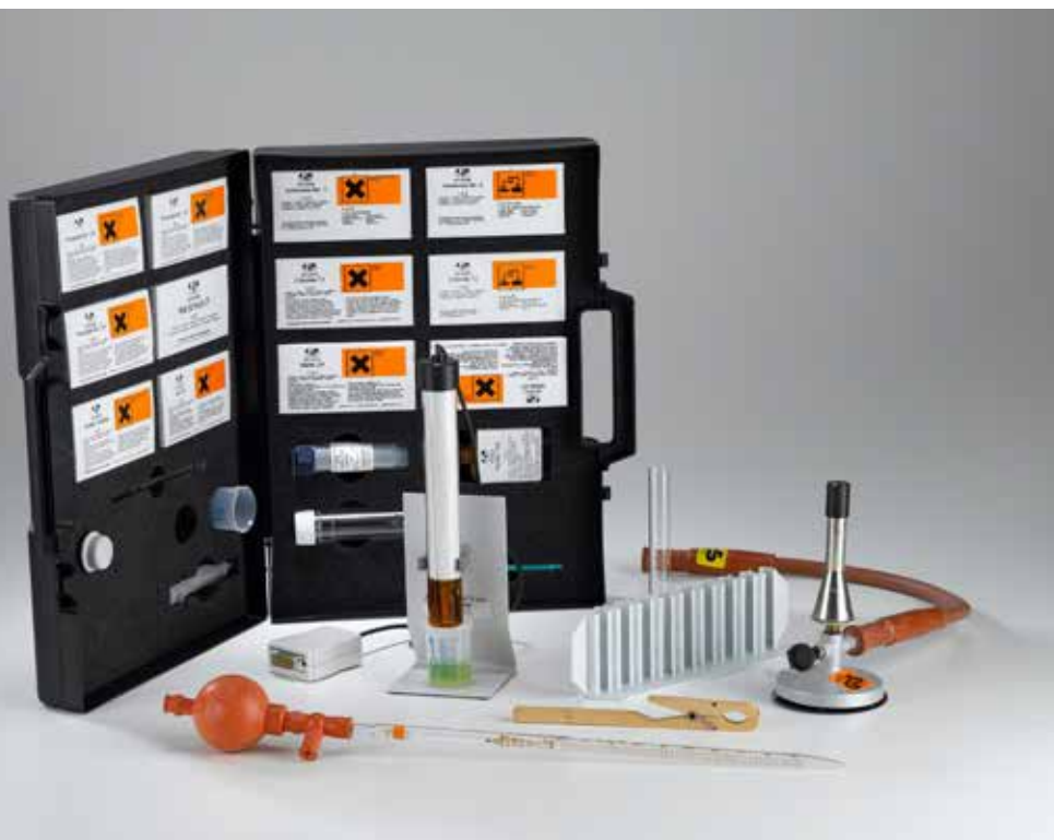
Determination of water contents with indicator reagents and immersion photometer (C3.6.1.1)
