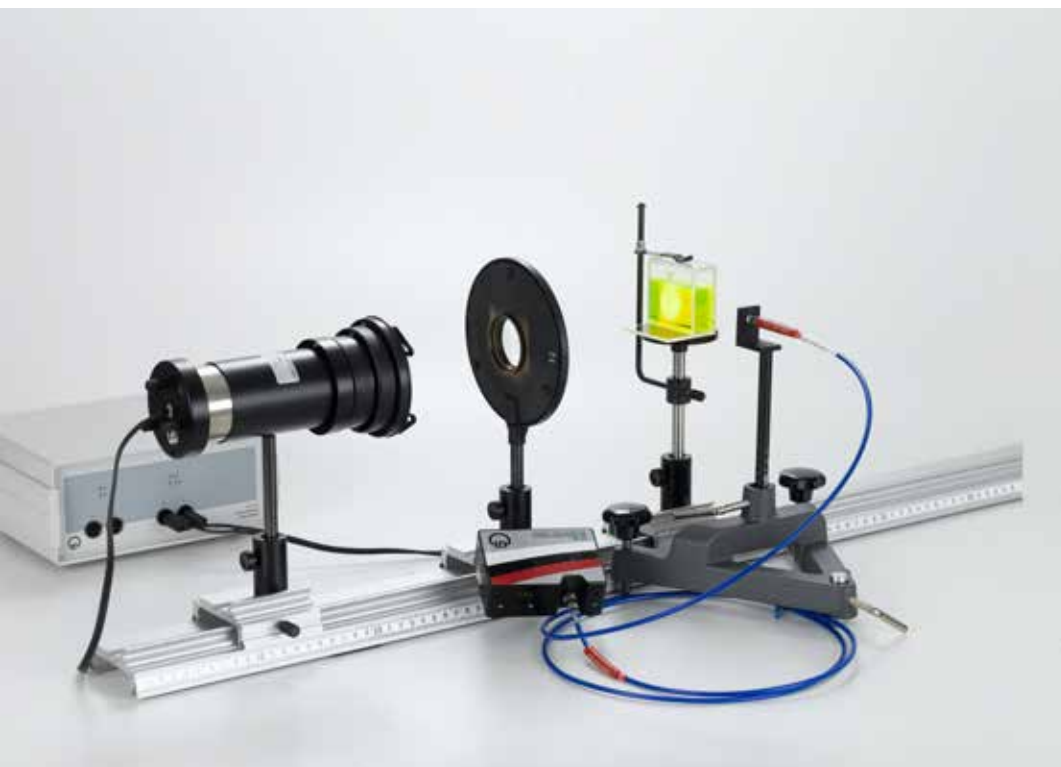
Recording of a fluorescence spectrum with a spectrometer (C3.3.1.3)
