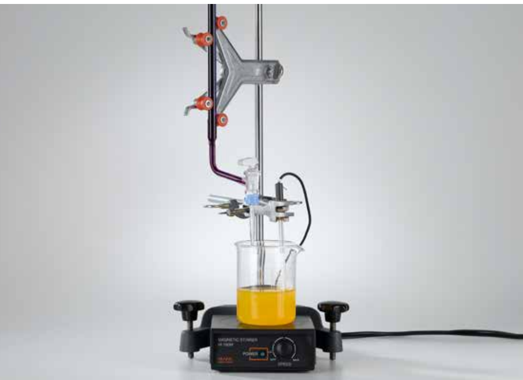
Manganometric determination of iron(II) ions (C3.5.3.2)
