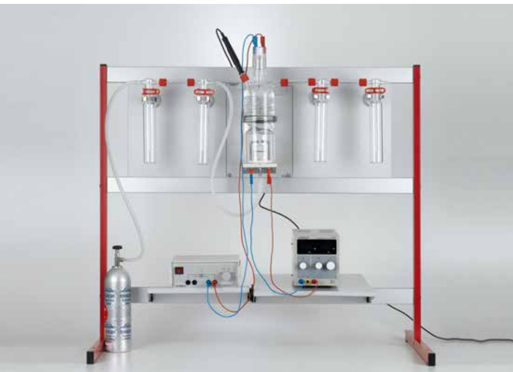
The calorific value of coal (C2.3.1.1)
