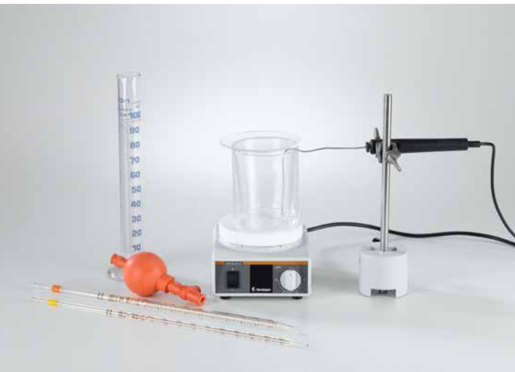
Determination of enthalpy of mixing (C4.3.3.4)
