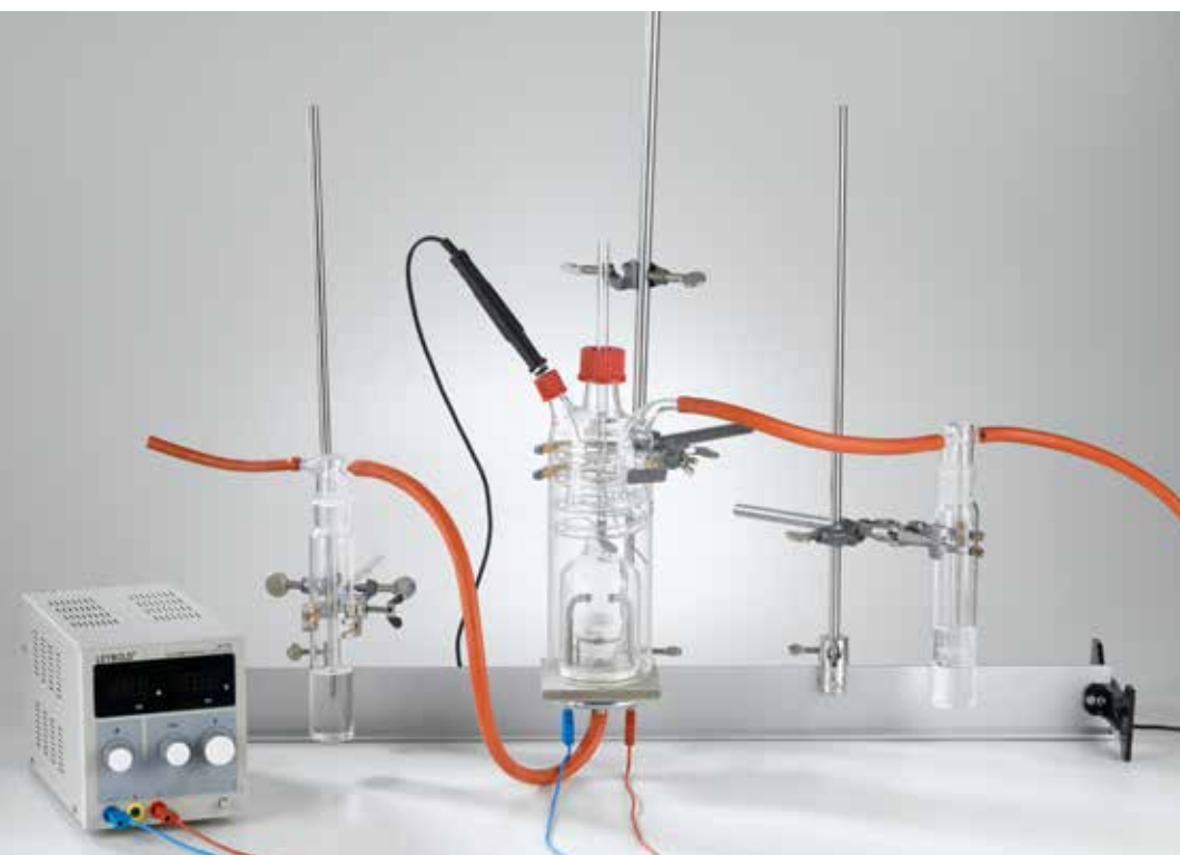
Determination of the calorific value of olive oil with a demonstration calorimeter (C6.1.4.1)
