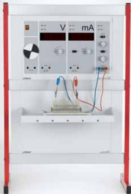
Determination of specific conductivity (C4.4.1.3)
