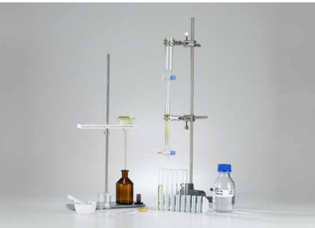
Separation of a leaf extract with column chromatography (C2.4.4.1)
