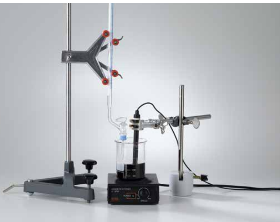
Determination of the content of phosphoric acid in a cola drink (C3.6.4.2)
