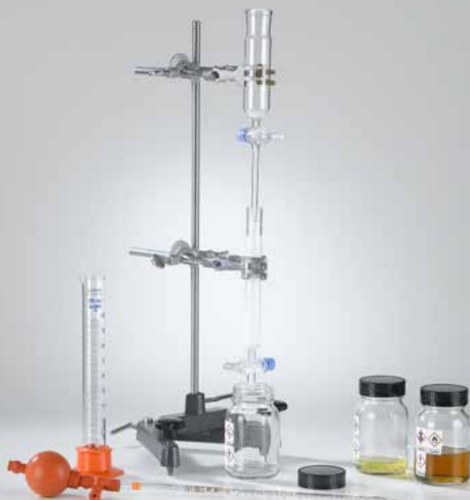
Separation of petroleum by means of column chromatography (C2.4.4.2)
