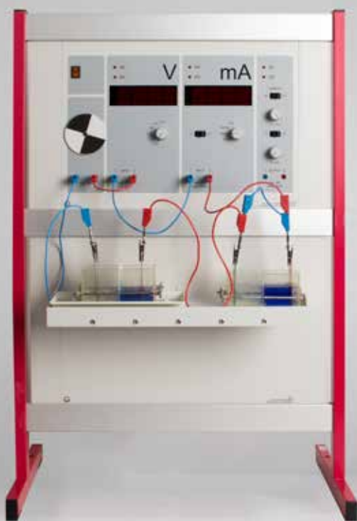
Serial and parallel connection of elements (C4.4.4.6)
