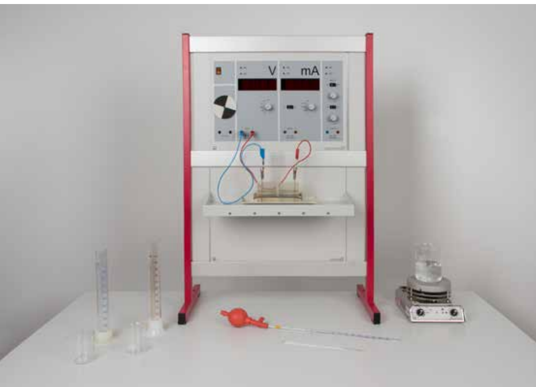
Temperature dependency of the potential (Nernst equation) (C4.4.3.5)
