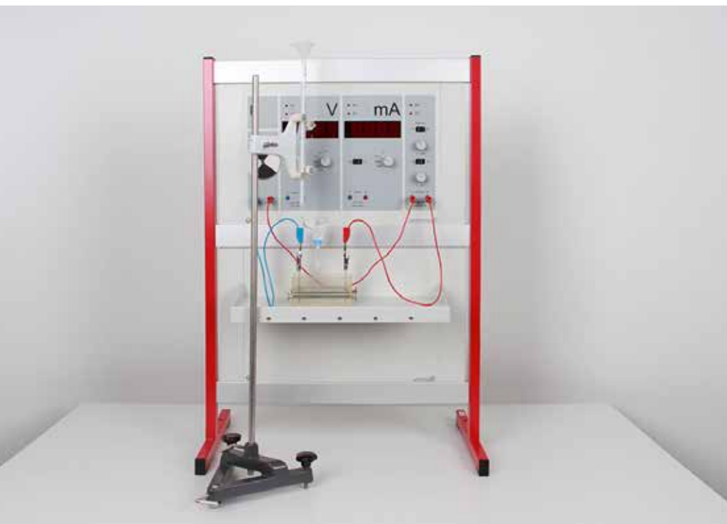
Conductometric titration using the Electrochemistry demonstration unit (C3.5.2.3)
