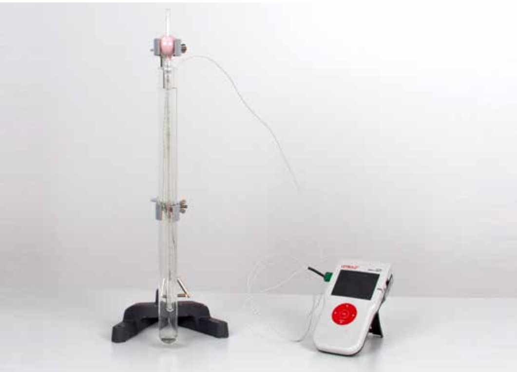
Temperature-dependency of the volume of a gas at a constant pressure (Gay-Lussac's law) (C1.4.4.2)
