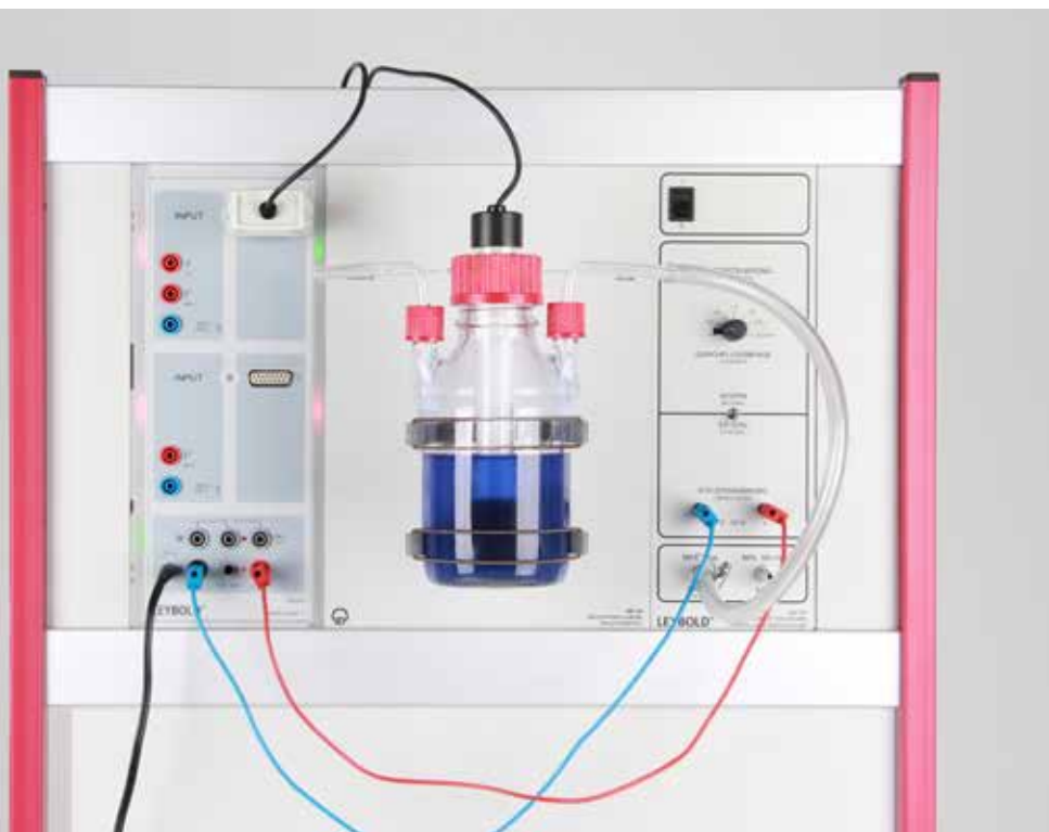
The automated Blue Bottle Experiment - a reversible redox reaction (C2.2.2.2)
