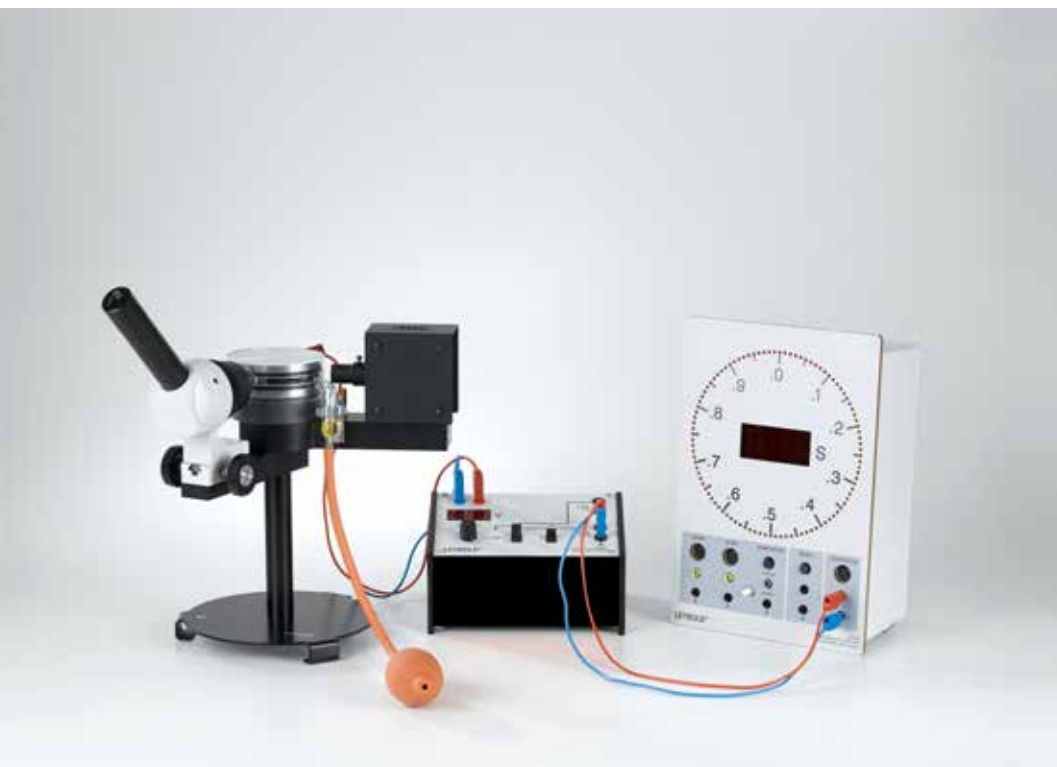
Determination of the elementary electric charge according to Millikan and proof of charge quantisation (C1.1.3.5)
