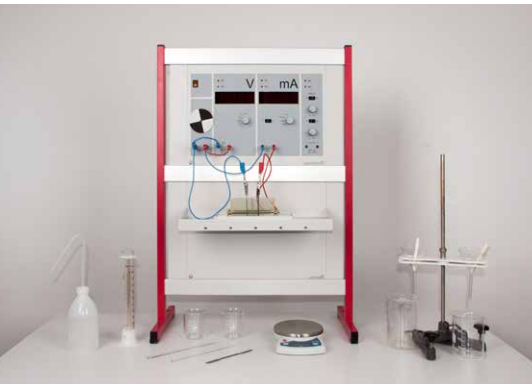
The Leclanché cell with Electrochemistry demonstration unit (C4.4.4.2_a)
