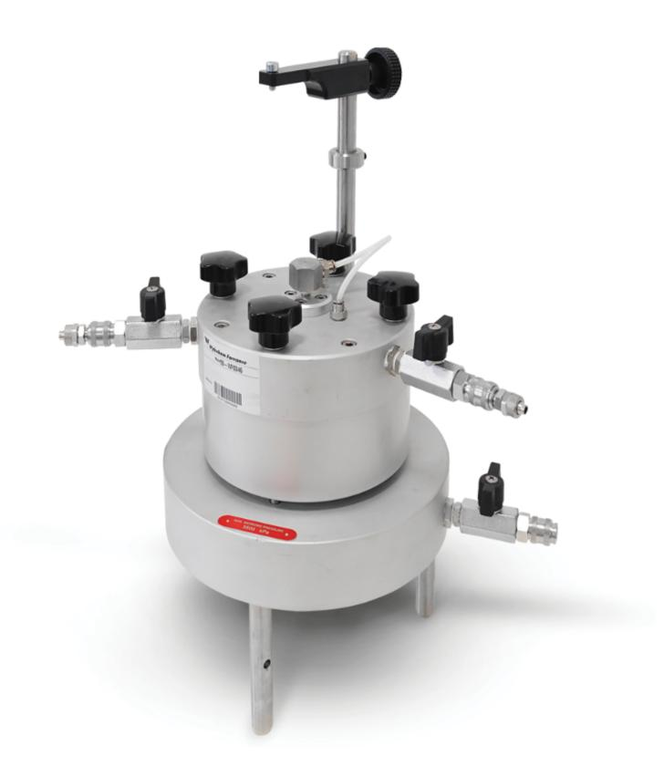
Used for hydraulic consolidation test on saturated soil sample.
