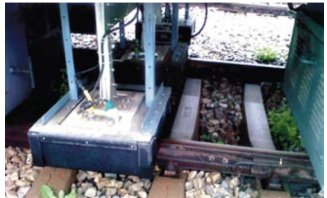
SRS configured with antennas beneath the train
