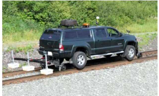
Road-rail vehicle equipped with SRS
